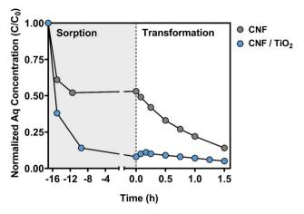
Fig. 5 Normalized aqueous (Aq) carbamazepine (CBZ) concentration  $(C/C_0; C_0 = 10 \mu M CBZ)$  over time during the sorption and electrochemical (EC) transformation periods. CBZ sorption was conducted in the dark, without an applied potential. The EC transformation was conducted at +1.00 V (vs. Ag/AgCl). Data are shown for the optimal composite (0.45 g PAN/50 wt% TiO<sub>2</sub>/1000 °C) and for CNFs without TiO<sub>2</sub> carbonized at 1000 °C.
