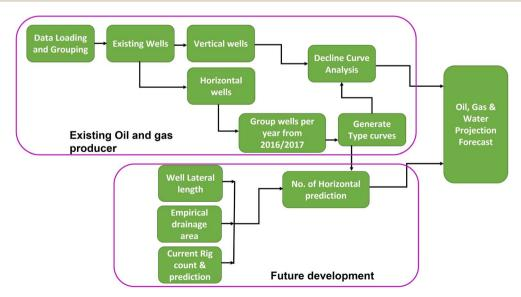
Workflow for a new systematic approach of forecasting net water production that can potentially be exported for beneficial reuse.
