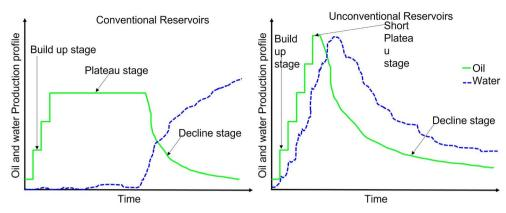
Fig. 6 Typical well oil and water production profiles for conventional and unconventional reservoirs
