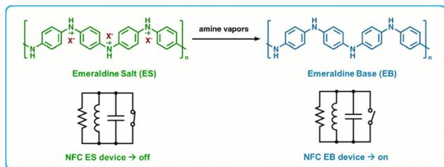
**Fig. 9** PTS-PAni based RFID amine sensors. Top: Chemical change of PTS-PAni upon exposure to amine vapors showing the transition from the Emeraldine Salt form to the Emeraldine Base form. Bottom: State change for NFC tags caused by the increase in resistance upon conversion to the Emeraldine Base form. Adapted with permission from Z. Ma, P. Chen, W. Cheng, K. Yan, L. Pan, Y. Shi and G. Yu, *Nano Lett.*, 2018, **18**, 4570–4575. Copyright 2018 American Chemical Society.<sup>140</sup>
