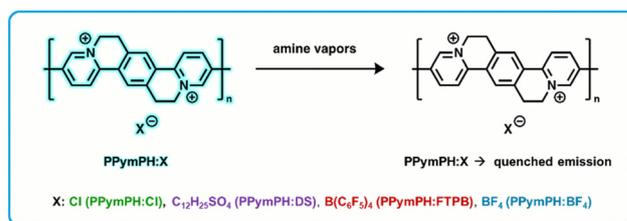
Fig. 5 PPymPh:X based “turn-off” fluorometric amine sensor exhibits analyte-induced emission quenching upon exposure to amine vapors.<sup>121</sup>
