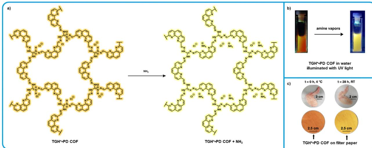
Fig. 7 TGH<sup>+</sup>·PD based “turn-on” fluorometric amine sensor. (a) Mechanism for the interaction of TGH<sup>+</sup>·PD with ammonia. (b) Modified images showing the resulting change in photoluminescence of TGH<sup>+</sup>·PD water dispersions from Trabolsi *et al.* (c) Modified images showing the color of TGH<sup>+</sup>·PD on filter paper after exposure to fresh and rotting chicken with permission from Trabolsi *et al.*<sup>127</sup>
