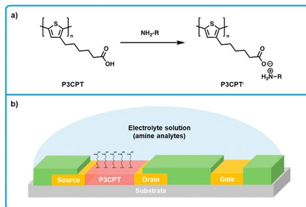
**Fig. 15** P3CPT based electrolyte-gated OTFT sensor for biogenic amines. (a) Mechanism for the interaction of P3CPT polymers and amine analytes showing a deprotonation of P3CPT. (b) Cross section showing the side-gate architecture used for the fabrication of OTFT sensors. Modified with permission from Minami *et al.*<sup>172</sup>
