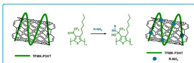
**Fig. 11** Diagram of TFMK-P3HT/CNT chemiresistors and the resulting addition reaction of amines to the trifluoromethyl ketone unit on TFMK-P3HT/CNT. Modified from Koo *et al* with permission in ref. 162
