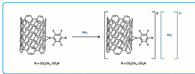
**Fig. 10** Diagram of chemiresistor sensing materials using a perfluorophenyl carboxylic acid functionalized SWCNT and the formation of a charge complex with ammonia.<sup>36</sup>
