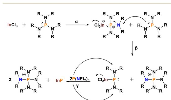
Scheme 2 Proposed mechanism for InP formation from  $P[In(Et)_2]_3$ .
