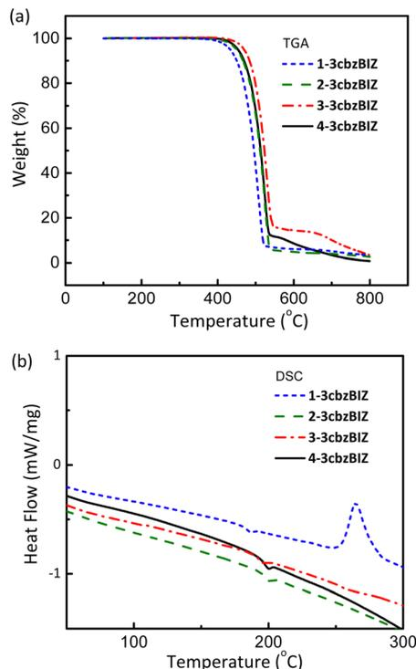
Fig. 2 (a) TGA curves; (b) DSC curves for **1-**, **2-**, **3-**, and **4-cbzBIZ**.
