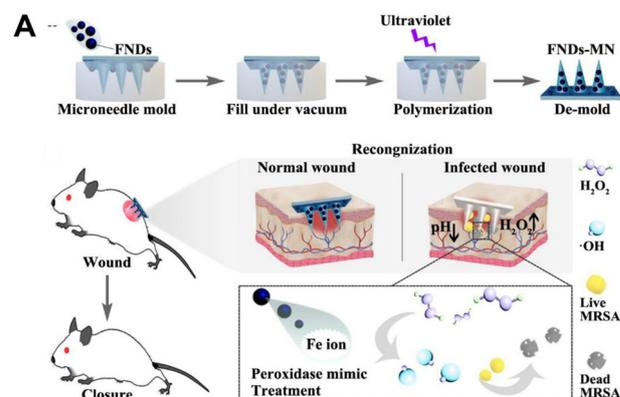
Fig. 3 (A) Schematic diagram of how the ligand polymer nanoparticle enzyme integrated colorimetric microneedle patches are made and how they are used to detect and treat wound infections.<sup>80</sup> Copyright 2022 Elsevier.
