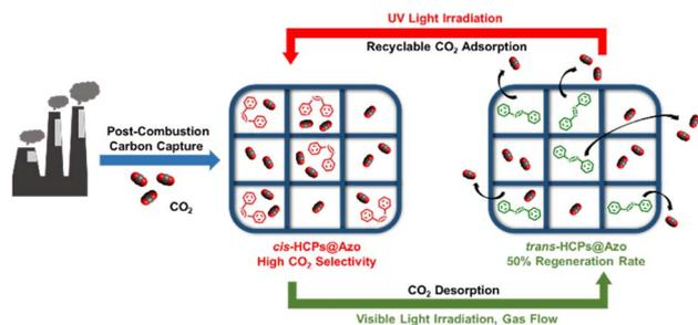
**Fig. 1** Our approach of exploiting photo-isomerisation of azobenzene molecules embedded in pores of HCPs to drive adsorption (upon UV irradiation) and desorption (vis-irradiation) of CO<sub>2</sub> to enable low-energy, low-cost carbon capture.
