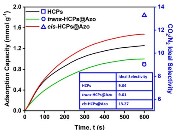
Fig. 3 CO<sub>2</sub> adsorption profiles of (black) HCPs, (green) visible light irradiated *trans*-HCPs@Azo and (red) UV light irradiated *cis*-HCPs@Azo using a flow rate of 10 mL min<sup>-1</sup>, pure CO<sub>2</sub> gas, at room temperature and atmosphere pressure. CO<sub>2</sub>/N<sub>2</sub> ideal selectivities of HCPs, *trans*-HCPs@Azo and *cis*-HCPs@Azo were obtained using CO<sub>2</sub> and N<sub>2</sub> pure gas adsorption capacities after 600 s (Table S2†).<sup>43,44</sup>
