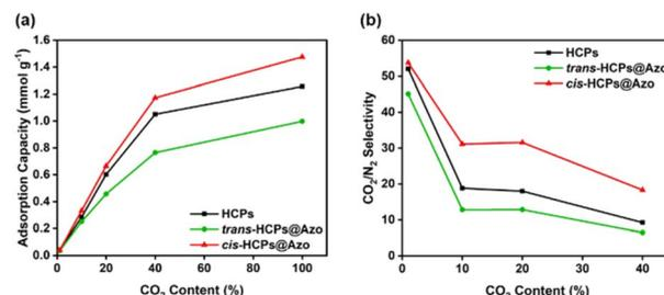
Fig. 4 (a) CO<sub>2</sub> adsorption capacities and (b) mixed gas CO<sub>2</sub>/N<sub>2</sub> selectivities (Table S3†)<sup>51,52</sup> of (black) HCPs, (green) *trans*-HCPs@Azo and (red) *cis*-HCPs@Azo at different CO<sub>2</sub> concentration of 1 v/v%, 10 v/v%, 20 v/v%, 40 v/v% and 100 v/v% at room temperature (25 °C) and atmosphere pressure (1 bar).
