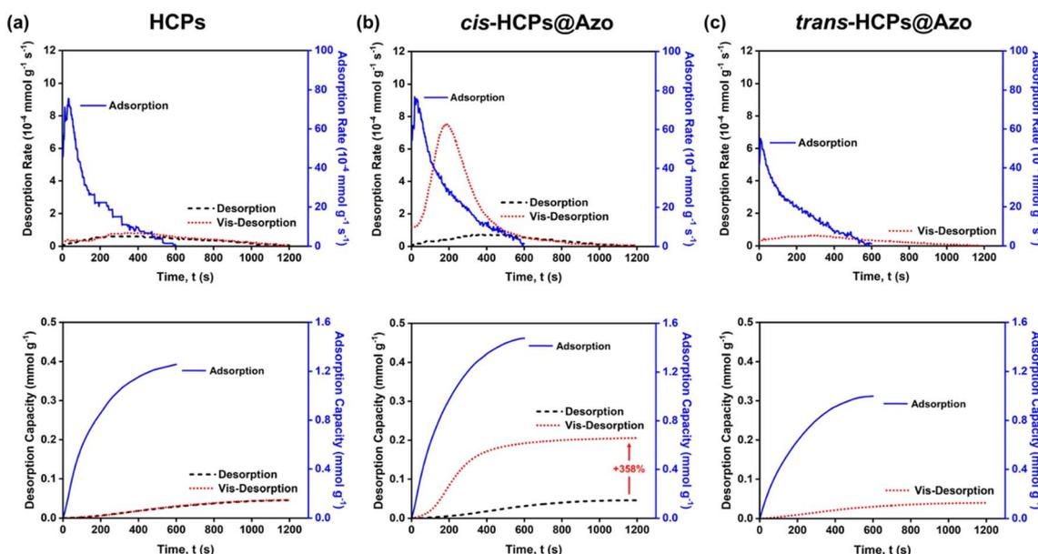
Fig. 5 The rate and capacities of adsorption (blue solid line) and desorption process (no visible irradiation: black dashed line; visible irradiation: red dotted line) of (a) HCPs, (b) *cis*-HCPs@Azo and *trans*-HCPs@Azo.
