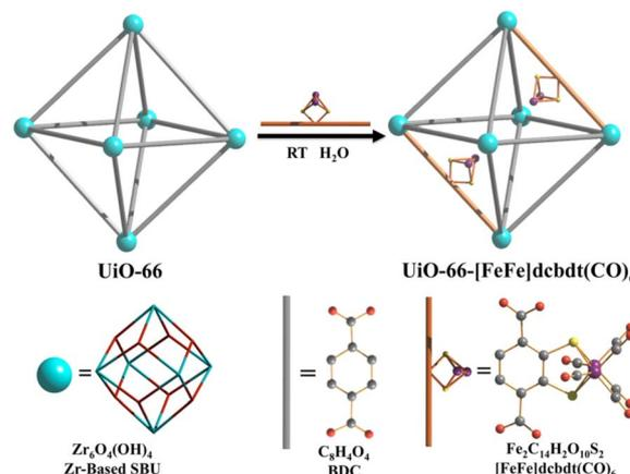
Fig. 4 Schematic representation of PSE of [FeFe](dcbdt)(CO)<sub>6</sub> into UiO-66. Reprinted from ref. 86 with permission from American Chemical Society (Copyright 2013).
