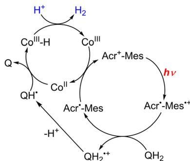
Scheme 20 Proposed mechanism of photocatalytic evolution of  $H_2$  from X-QH<sub>2</sub> with  $Acr^+ - Mes$  and  $Co^{III}(dmgH)_2ClPy$ . Reprinted from ref. 164 with permission from American Chemical Society (Copyright 2020).
