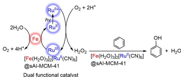
Scheme 3 Photocatalytic cycle for PhOH production from  $\text{C}_6\text{H}_6$  and  $\text{O}_2$  with  $[\text{Fe}(\text{II})(\text{H}_2\text{O})_3]_2[\text{Ru}(\text{II})(\text{CN})_6]$ @sAl-MCM-41.<sup>76</sup>
