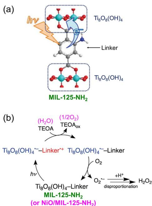
Scheme 11 Visible light-driven  $2e^- \text{O}_2$  reduction to  $\text{H}_2\text{O}_2$  with TEOA catalyzed by Ni/MIL-125- $\text{NH}_2$ . Reproduced from ref. 96 with permission from the Royal Society of Chemistry (Copyright 2018).
