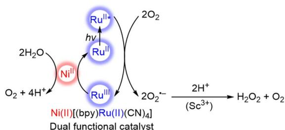
Scheme 2 Catalytic mechanism for the formation of hydrogen peroxide from water and dioxygen with a dual functional catalyst,  $Ni(II)((bpy)Ru(II)(CN)_4)$ , under visible light irradiation.<sup>71</sup>
