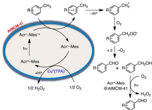
**Scheme 15** Photocatalytic mechanism for the oxidation of *p*-xylene selectively by  $O_2$  with  $[Cu(II)(TPA)]^{2+}/Acr^+-Mes@AIMCM-41$ . Reprinted from ref. 122 with permission from the National Academy of Sciences (Copyright 2012).
