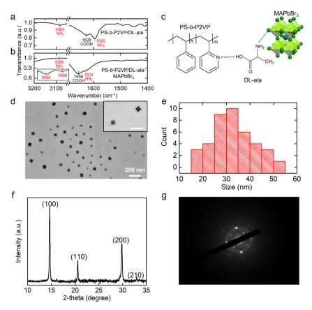
Fig. 2 FTIR spectra of (a) PS-b-P2VP/DL-ala and (b) PS-b-P2VP/DL-ala inverse micelle-encapsulated MAPbBr<sub>3</sub> NCs. (c) Molecular structures showing the chemical interactions among PS-b-P2VP, DL-ala, and MAPbBr<sub>3</sub> NCs. (d) TEM image (inset: high-magnification TEM image, scale bar: 100 nm), (e) size distribution histogram (average size: 32.7 nm), (f) XRD pattern, and (g) the SAED pattern of the PS-b-P2VP/DL-ala inverse micelleencapsulated MAPbBr3 NCs.
