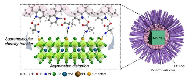
Fig. 4 Proposed mechanism for the origin of chirality in the PS-b-P2VP/DL-ala inverse micelle-encapsulated MAPbBr<sub>3</sub> NCs, illustrating that the P2VP/pL-ala chains passivating the NC surfaces cause asymmetric surface lattice distortions.
