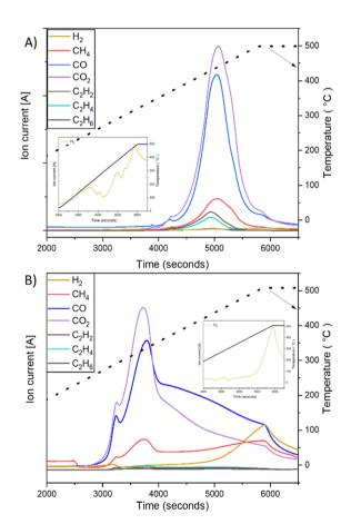
Fig. 2 Gas evolution profile for catalytic pyrolysis experiment (with zoom of H<sub>2</sub> evolution). (A) PET and (B) cotton.
