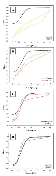
Fig. 2 Comparison between voltammograms of graphite (black line) and biochar electrodes obtained at different temperatures: 500 °C (A), 600 °C (B), 800 °C (C), and 1000 °C (D) in a single chamber three electrode electrochemical cell with G. sulfurreducens already grown. Cyclic voltammetry was performed at 0.001 V s<sup>-1</sup> and current density divided by maximal current density  $(j/j_{max})$  vs. potential (E/V) is plotted in the y axis.
