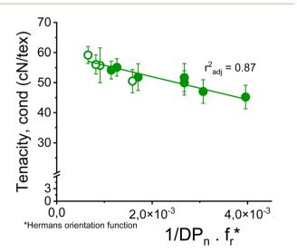
Fig. 13 Conditioned tenacity of loncell fibers with titers of  $1.21\pm0.10$  dtex made from SWS-IP (open circles) and HWPHK pulps (closed circles) as a function of the reciprocal DP $_n$  times the Hermans orientation function  $f_r$ .
