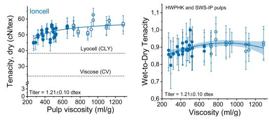
Fig. 10 Strength properties of the spun fiber as a function of pulp viscosity. Left: conditioned tenacity, right: ratio between conditioned and wet tenacities (closed circles: HWPHK pulps; open circles: SWS-IP pulps).
