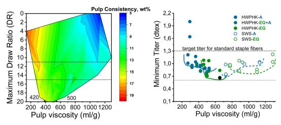
Fig. 7 Effect of pulp viscosity and dope concentration on the maximum filament draw ratios (left) and the effect of pulp viscosity on the minimum titer of the spun fiber (right).
