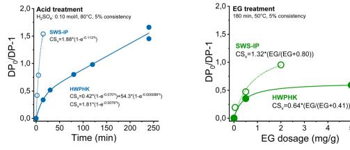
Fig. 1 The chain scission rate of cellulose during the acid (left) and endoglucanase treatment (right).
