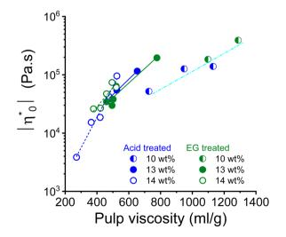
Fig. 4 Relationship between dope zero shear viscosity and pulp viscosity for the dope concentrations 10, 13 and 14 wt%.
