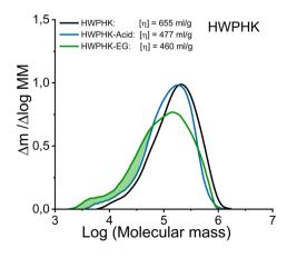
Fig. 2 Molecular mass distribution of the acid and enzyme-treated SWS-IP (left) and HWPHK pulps (right).
