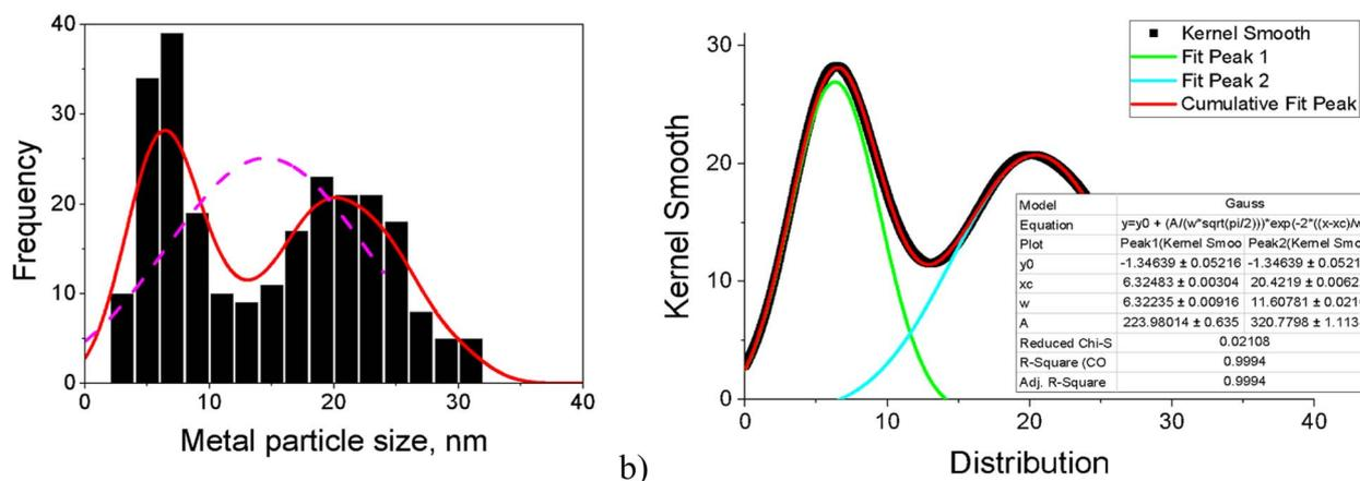
**Fig. 2** (a) Histogram of the FeNi particle size and (b) fitting curves of kernel smooth distribution for the spent catalyst after dihydrogenol hydrodeoxygenation in the batch reactor (Table 1, entry 2).
