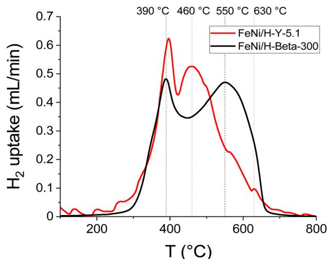
Fig. 7  $H_2$ -TPR profiles of the fresh catalyst: 5–5 wt% Fe–Ni/H–Y–5.1 (data from ref. 12) and 5–5 wt% Fe–Ni/H–Beta–300.
