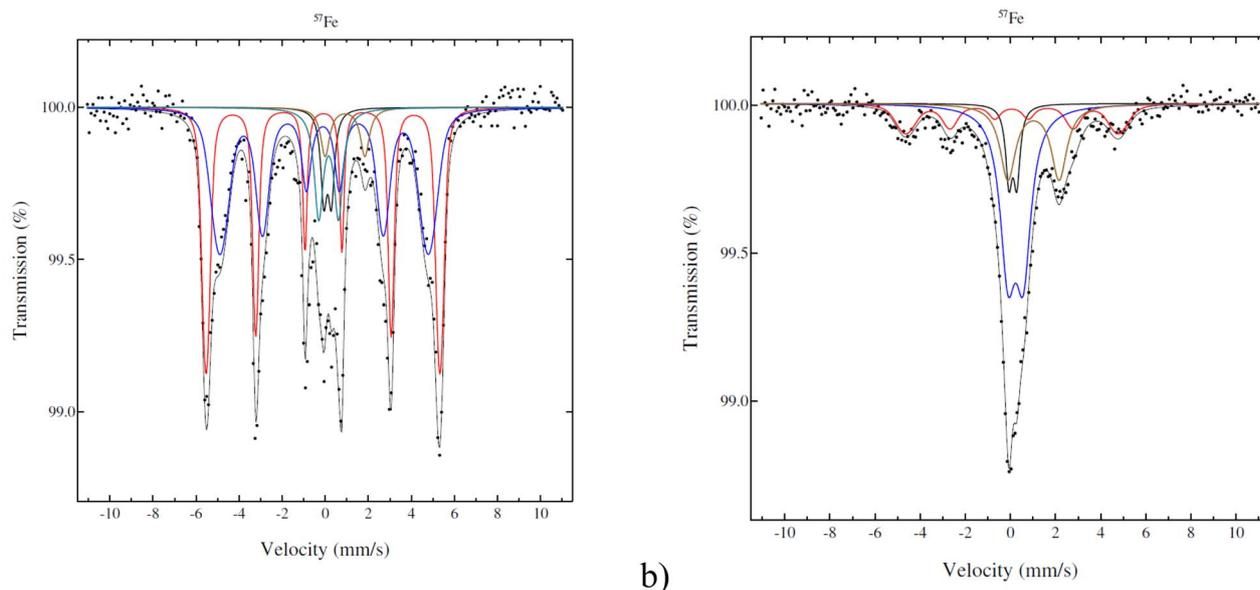
Fig. 4 Mössbauer spectra of the fresh catalyst: (a) 5–5 wt% Fe–Ni/H–Beta–300, legend: metallic and magnetic Fe (red, blue),  $\text{Fe}^{2+}$  (brown),  $\text{Fe}^{3+}$  (cyan), Fe impurity in the detector (black); (b) 5–5 wt% Fe–Ni/H–Y–5.1,<sup>12</sup> legend: metallic and magnetic Fe (red),  $\text{Fe}^{2+}$  (beige),  $\text{Fe}^{3+}$  (blue), Fe impurity in the detector (black).
