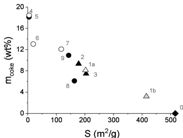
Fig. 9 Amount of coke determined by TGA as a function of the catalyst-specific surface area. Legend: fresh catalyst (diamond), spent catalyst from the batch experiment (triangle), spent catalyst from the continuous experiments (circle), spent catalyst from IE HDO (open symbols) and spent catalyst from DHE HDO (black symbols), regenerated catalyst (grey symbol, *in situ* regeneration of the spent catalyst simulated by O<sub>2</sub>-TPO). Notation is the same as in Table 4.
