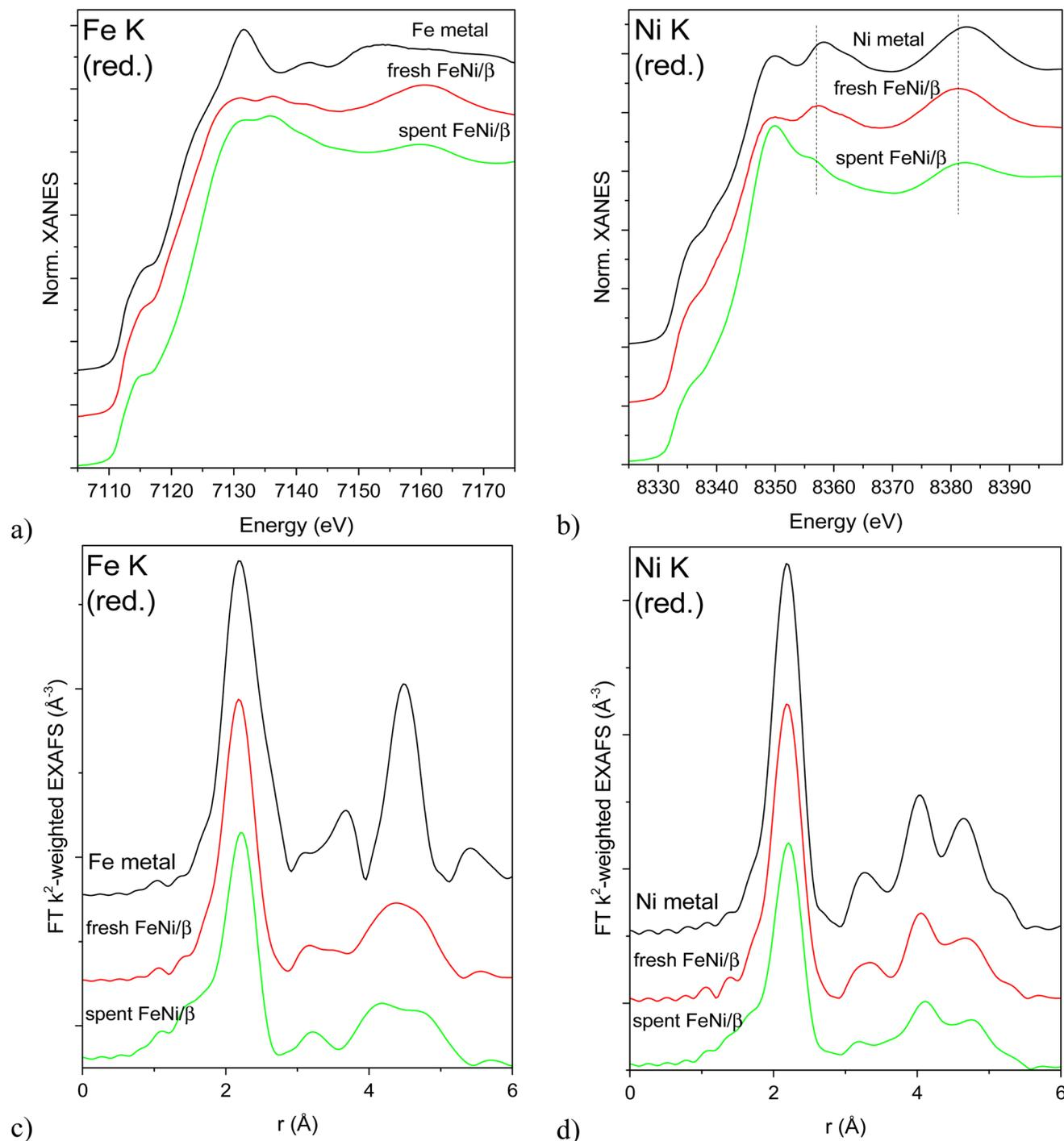
Fig. 6 Normalized XANES (a and b) and Fourier transformed EXAFS (c and d) spectra of reduced fresh and re-reduced spent catalysts and the respective bulk metals (5  $\mu\text{m}$  thick foils) measured at Fe K (a and c) and Ni K (b and d) edges. EXAFS spectra are not corrected for the phase shift.
