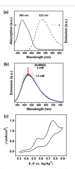
Fig. 2 (a) UV-vis absorption (solid) and emission (dash) spectra of DPTC in acetonitrile. Emission spectrum was obtained with excitation at  $\lambda_{\rm ex}=380$  nm. (b) Emission quenching for DPTC with KABNO (conc. =0-1.2 mM). (c) CV of KABNO and LMC in 0.1 M TBAPF $_6$  acetonitrile solution. The experiment was performed using a glassy carbon working electrode, Pt counter electrode, and Ag/Ag $^+$  reference electrode in the dark.
