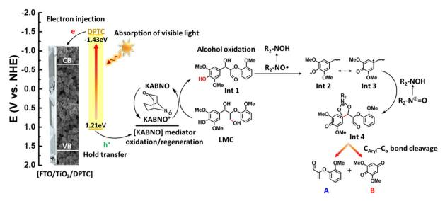
Fig. 6 Proposed mechanism for oxidative C–C bond cleavage to give products **A** and **B** in the DSPEC system by using the FTO/TiO $_2$ /DPTC photoanode and KABNO ( $R_2$ NO $^*$ ) in the presence of LMC.
