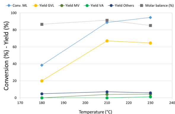
Fig. 1 Effect of temperature on ML hydrogenation over Re–O/HZSM-5. Reaction conditions: solvent free (ML neat), T = variable, P_{H_2} = 40 bar, t = 4 h, catalyst loading = 5 wt% [ m_{cat}/m_{ML} ]. Others = 2-MTHF, 4-HPA/E and unidentified products.
