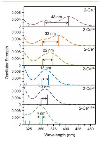
Fig. 5 TD-DFT spectra accentuating the splitting between the higher and lower energy 4f-5d transitions in the  $Ce^{3+}$  complexes. Vertical bars depict the theoretical oscillator strength of single-electron excitations. Half-width at half height is 0.15 eV.
