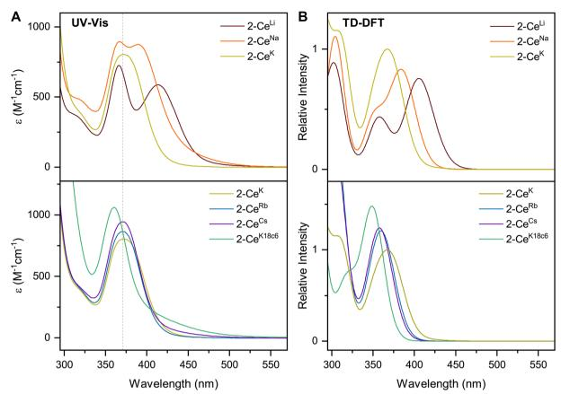
Fig. 4 (A) Experimental UV-vis spectra measured in toluene, except for **2-Ce<sup>K18c6</sup>**, which was measured in THF. (B) Calculated spectra from TD-DFT, with half width at half height at 0.15 eV. Direct comparison of TD-DFT and UV-vis spectra for each complex is shown separately in Fig. S92–S99.†
