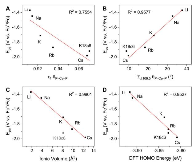
Fig. 3  $E_{\rm pa}$  measured by cyclic voltammetry (50 mM [ $^n$ Bu<sub>4</sub>N][BPh<sub>4</sub>] in THF) plotted vs. (A)  $\tau_4$  calculated using P–Ce–P angles. (B)  $\Sigma_{\Delta 109.5}$  calculated using P–Ce–P angles. (C) Ionic volume (4/3· $\pi r^3$ , r= Shannon ionic radius<sup>39</sup>), 2-Ce<sup>K18c6</sup> data excluded from linear regression analysis. (D) Computed HOMO energy levels.
