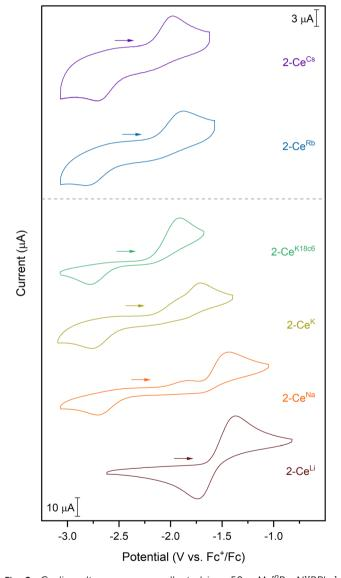
Fig. 2 Cyclic voltammograms collected in a 50 mM [ $^nBu_4N$ ][BPh $_4$ ] solution in THF. Analyte concentration is 3 mM for all complexes, except for  $2\text{-Ce}^{Rb}$  and  $2\text{-Ce}^{Cs}$ , which were measured at 1 mM analyte concentration.
