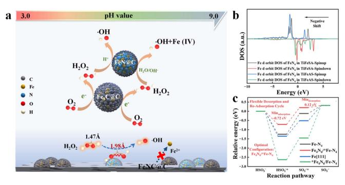
Fig. 1 Probable role of Fe<sub>3</sub>C and FeN nanoparticles in the FeNC@C catalyst for enhanced heterogeneous electro-Fenton performance, reprinted (adapted) with permission from ref. 2 copyright 2021 ACS. (b) The Fe d orbit DOS of FeN₄ in TiFeSA and TiFeAS. (c) Reaction energy diagrams for PMS oxidation on  $Fe-N_4$ ,  $Fe_4N_6$ /\* $FeN_4$ , Fe[111], and \* $Fe_4N_6$ / $FeN_4$ , reprinted (adapted) with permission from ref. 1. Copyright 2023 PNAS.
