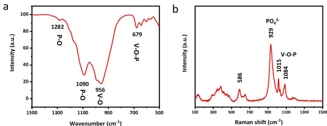
Fig. 2 (a) FTIR spectra and (b) Raman spectra of  $\delta$ -VOPO<sub>4</sub> powder.
