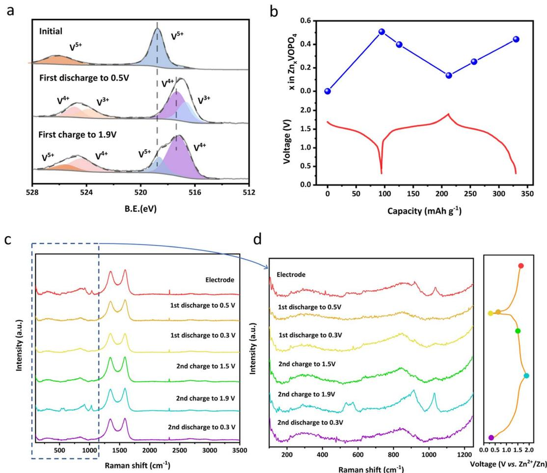
Fig. 4 (a) *Ex situ* XPS spectra of V 2p of  $\delta$ -VOPO<sub>4</sub>; (b) *ex situ* ICP measurement of  $\delta$ -VOPO<sub>4</sub> during the first two cycles; (c and d) *ex situ* Raman spectra of  $\delta$ -VOPO<sub>4</sub> during the first two cycles.
