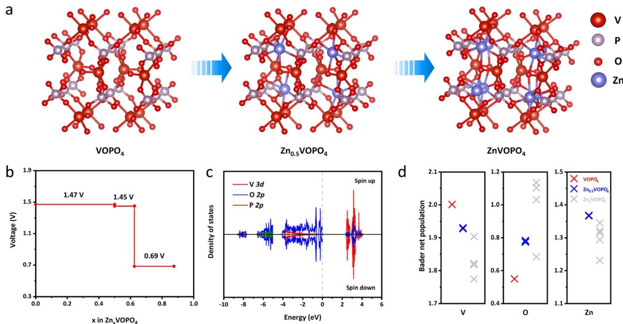
Fig. 5 (a) The schematic illustration of structural models of  $\delta$ -VOPO<sub>4</sub> before and after dezincification; (b) the equilibrium reaction voltage profiles predicted with DFT calculations; (c) the density of states (DOS) of  $\delta$ -VOPO<sub>4</sub>; the Fermi energy level is set to zero; (d) the Bader charge analysis of  $\delta$ -VOPO<sub>4</sub>.
