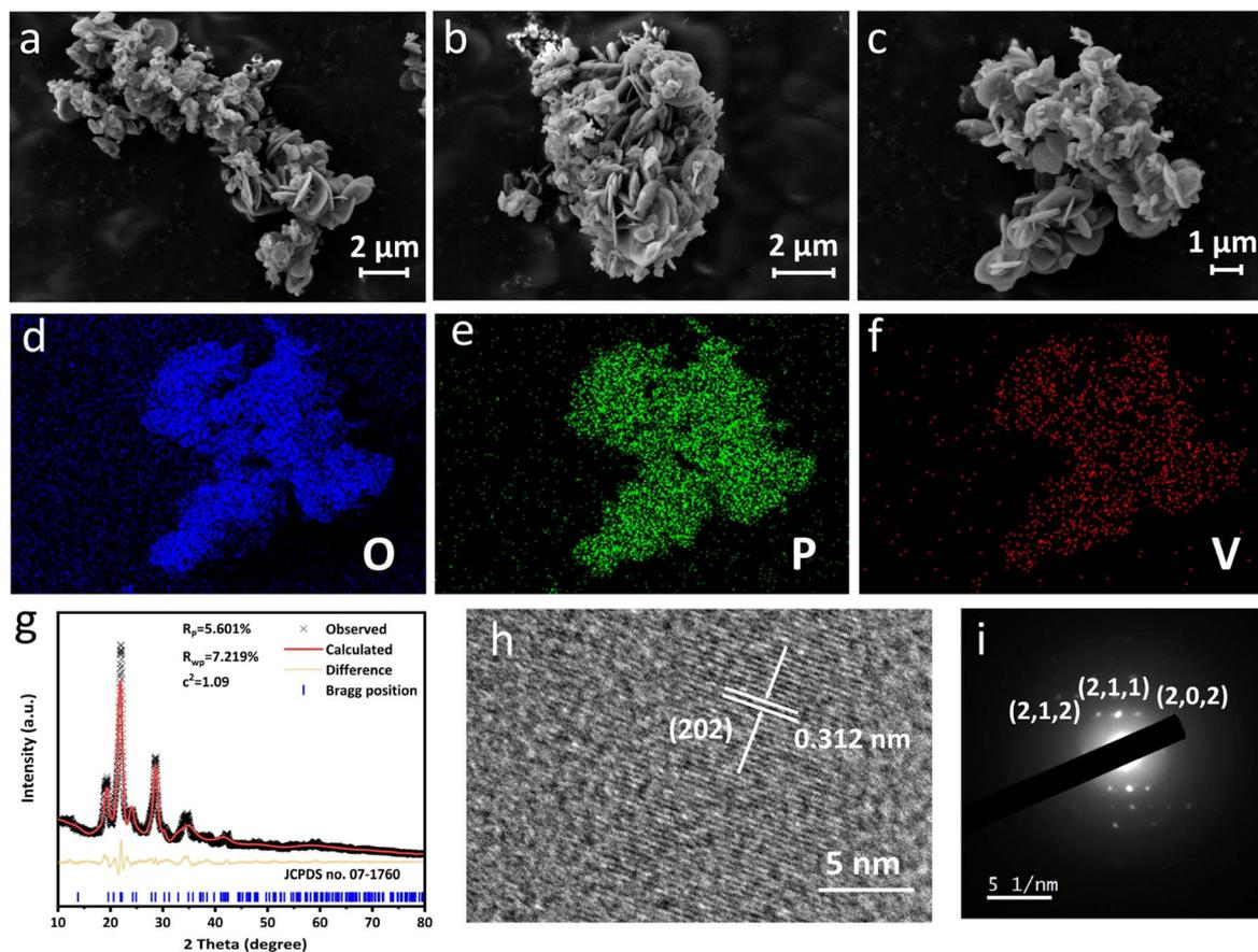
Fig. 1 (a–c) SEM images, (d–f) elemental mappings, (g) Rietveld XRD pattern, (h) HR-TEM and (i) SAED images of  $\delta$ -VOPO<sub>4</sub>.
