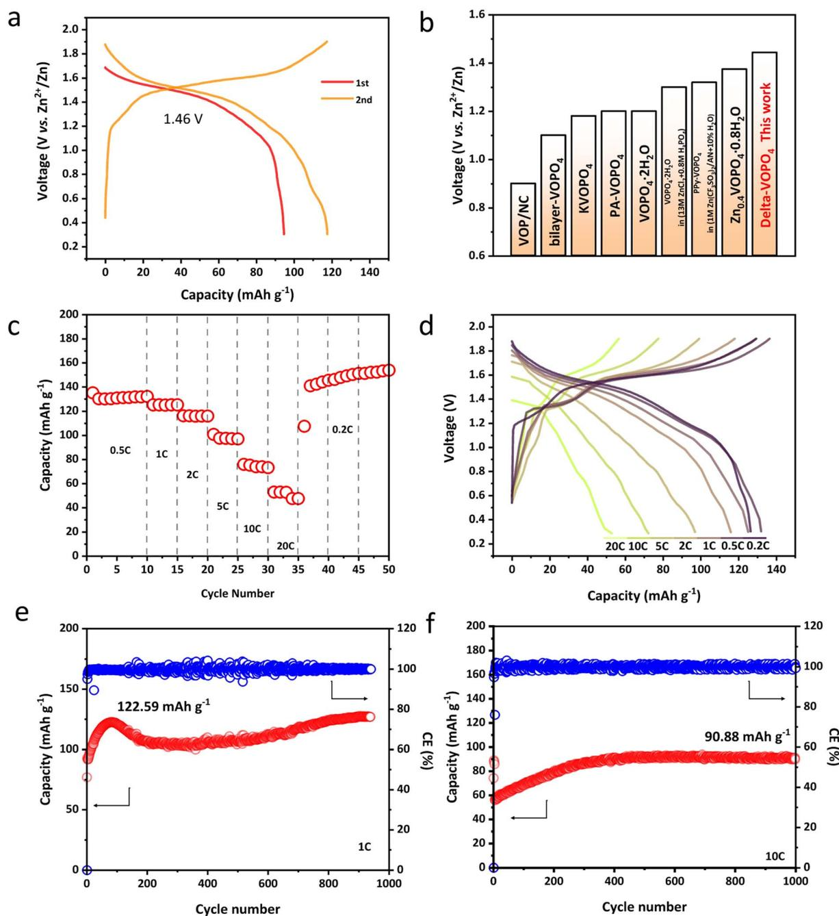
Fig. 3 (a) The first two discharge/charge curves of  $\delta$ -VOPO<sub>4</sub>; (b) the average discharge voltage of reported VOPO<sub>4</sub> materials<sup>13–17,37,38</sup> and this work; (c) rate performances of  $\delta$ -VOPO<sub>4</sub> at different current densities; (d) charge/discharge curves of  $\delta$ -VOPO<sub>4</sub> at different current densities; cycling performance of  $\delta$ -VOPO<sub>4</sub> at 1C (330 mA g<sup>-1</sup>) (e) and 10C (3300 mA g<sup>-1</sup>) (f).
