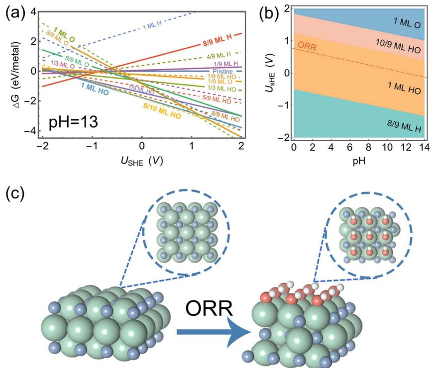
Fig. 1 (a) Calculated 1D surface Pourbaix diagram as a function of potential (vs. SHE) ( $\text{pH} = 13$ ;  $T = 298.15 \text{ K}$ ). (b) 2D surface Pourbaix diagram as a function of potential (vs. SHE) and  $\text{pH}$  ( $T = 298.15 \text{ K}$ ). (c) Optimized structures of the ZrN(100) surface before and after  $\text{HO}^*$  coverage under ORR conditions. Insets are the corresponding top views. Green, blue, red, and white spheres denote Zr, N, O, and H, respectively.
