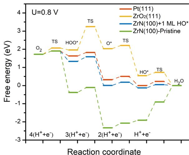
Fig. 2 Calculated free energy diagrams of the ORR at pristine ZrN(100) and ZrN(100) covered by 1 ML  $\text{HO}^*$ , Pt(111),<sup>40</sup> and  $\text{ZrO}_2(111)$ .<sup>19</sup> The energy barriers of the elementary steps were estimated based on the method by Dickens *et al.*<sup>41</sup> The potential was set to 0.8 V vs. RHE.
