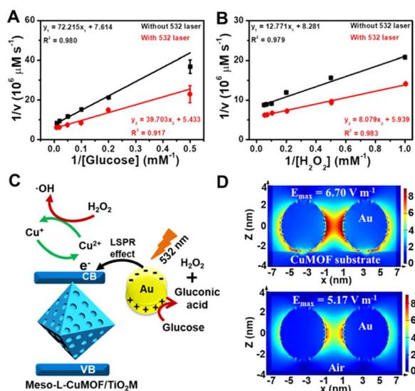
Fig. 4 Lineweaver–Burk plot of Au@Meso-L-CuMOF/TiO<sub>2</sub>M for the changes in (A) glucose and (B) H<sub>2</sub>O<sub>2</sub> in the presence and absence of 532 nm irradiation. (C) Schematic illustration of surface plasmon-enhanced nanoenzyme activity under 532 nm irradiation. (D) The intensity of electric field distribution in the monitor window around the hotspot on Au/CuMOF and Au NPs.
