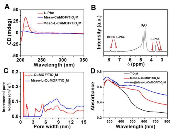
Fig. 2 (A) CD spectra of Meso-L-CuMOF/TiO<sub>2</sub>M, L-Phe, and Meso-L-CuMOF/TiO<sub>2</sub>M. (B) Liquid <sup>1</sup>H NMR spectrum of Meso-L-CuMOF/TiO<sub>2</sub>M digested in D<sub>2</sub>O. (C) Pore size distribution of Meso-L-CuMOF/TiO<sub>2</sub>M before and after CTAB removal. (D) Absorption spectra of TiO<sub>2</sub>M, Meso-L-CuMOF/TiO<sub>2</sub>M, and Au@Meso-L-CuMOF/TiO<sub>2</sub>M.
