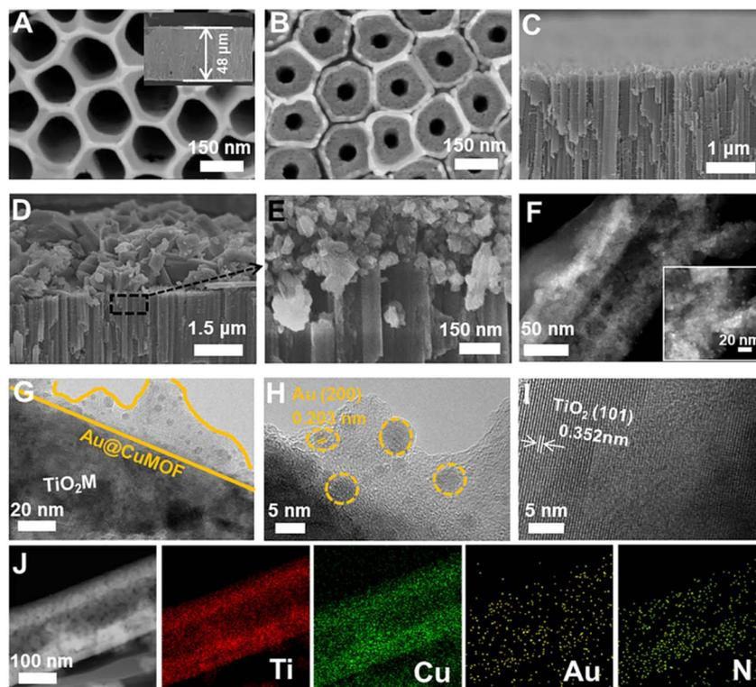
Fig. 1 Schematic illustration of preparing Au@Meso-L-CuMOF/TiO<sub>2</sub>M. SEM images: (A) top view, (B) bottom view, and (C) side view of TiO<sub>2</sub>M. (D and E) Side view of Meso-L-CuMOF/TiO<sub>2</sub>M. (F) HAADF-STEM, (G) TEM and (H and I) HRTEM images of Au@Meso-L-CuMOF/TiO<sub>2</sub>M. (J) Elemental mapping of Au@Meso-L-CuMOF/TiO<sub>2</sub>M.
