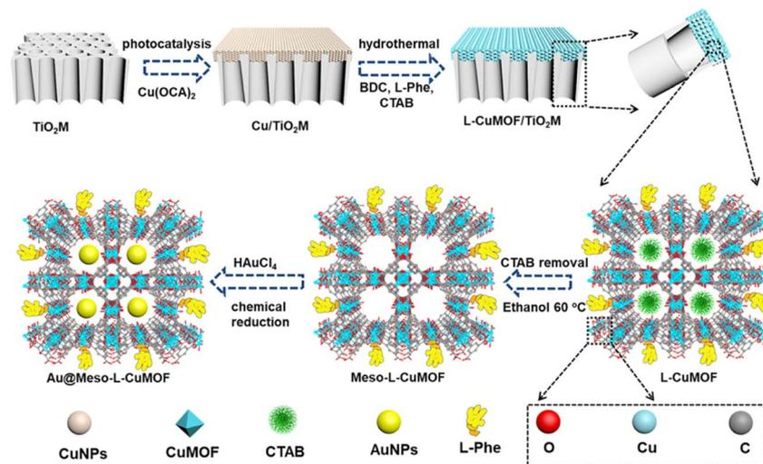
Scheme 1 Schematic illustration of preparing Au@Meso-L-CuMOF/TiO<sub>2</sub>M from TiO<sub>2</sub>M.
