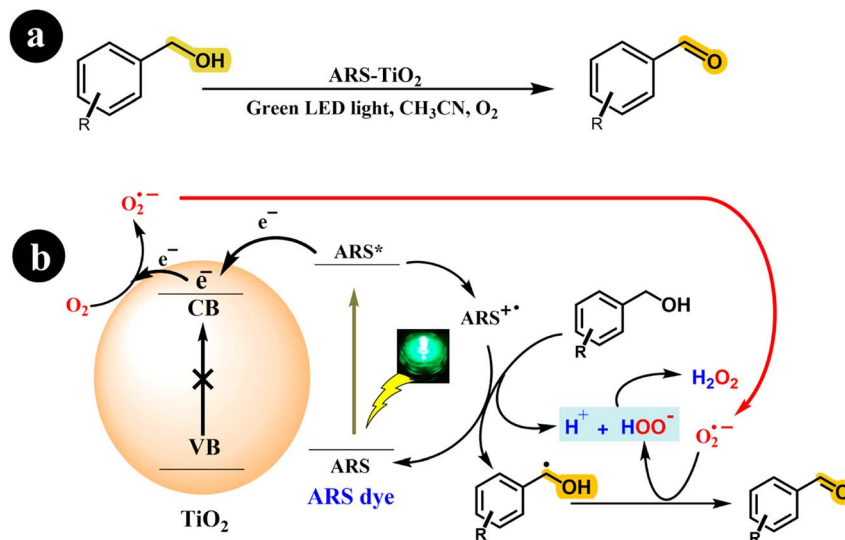
Scheme 4 (a) The reaction conditions and (b) the proposed mechanism for the selective oxidation of benzyl alcohol with air using dye-sensitized \text{TiO}_2 photocatalysis under visible light irradiation. Reproduced with permission from ref. 38, copyright 2018, Elsevier.
