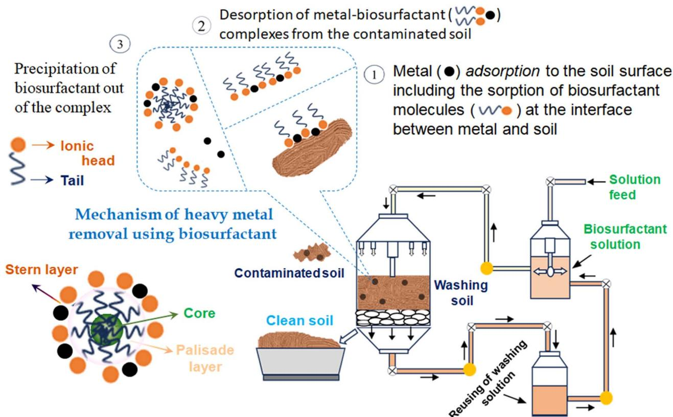
**Fig. 8** Technique for heavy metal removal from contaminated soil using biosurfactants and the obtained removal rates for Cu, Zn, Cr, and Cd of 90–100% in normal conditions.
