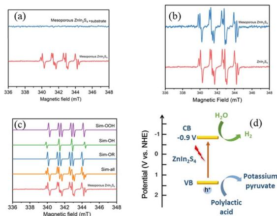
Fig. 8 EPR spectra of free radicals captured by DMPO of (a) mesoporous  $\text{ZnIn}_2\text{S}_4$  under simulated solar light with or without substrate; (b) mesoporous  $\text{ZnIn}_2\text{S}_4$  and  $\text{ZnIn}_2\text{S}_4$  under simulated solar light without substrate (c) simulation of EPR spectra of free radicals captured by DMPO of mesoporous  $\text{ZnIn}_2\text{S}_4$ ; (d) proposed mechanism for photoreforming of PLA by mesoporous  $\text{ZnIn}_2\text{S}_4$ .
