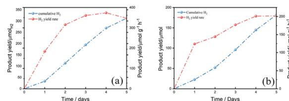
Fig. 7 Long-term photoreforming of (a) PLA and (b) PET. Reaction conditions: photocatalyst (1.5 mg mL<sup>-1</sup>), pretreated polymers (25 mg mL<sup>-1</sup>), aqueous KOH (1 M, 5 mL), and simulated sunlight (AM 1.5 G, 150 mW cm<sup>-2</sup>, rt).
