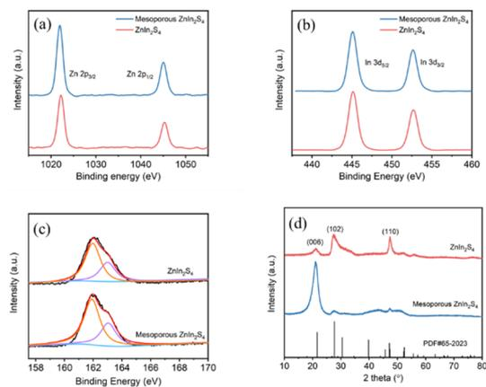
Fig. 2 (a) Zn 2p, (b) In 3d, and (c) S 2p XPS spectra of  $\text{ZnIn}_2\text{S}_4$  and mesoporous  $\text{ZnIn}_2\text{S}_4$ . (d) XRD profiles of  $\text{ZnIn}_2\text{S}_4$  and mesoporous  $\text{ZnIn}_2\text{S}_4$ .
