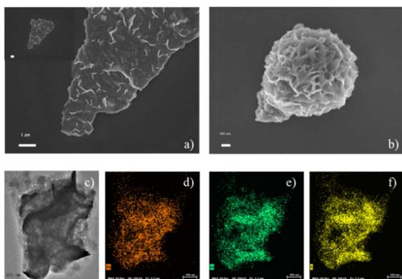
Fig. 1 SEM images of (a) mesoporous  $\text{ZnIn}_2\text{S}_4$  and (b)  $\text{ZnIn}_2\text{S}_4$ ; TEM image of (c) mesoporous  $\text{ZnIn}_2\text{S}_4$  and (d) Zn, (e) In and (f) S atom element mapping of mesoporous  $\text{ZnIn}_2\text{S}_4$ .
