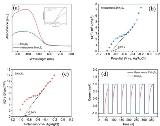
Fig. 4 (a) UV-vis DRS, inset: Tauc plot of samples; Mott-Schottky curves of (b) mesoporous  $\text{ZnIn}_2\text{S}_4$  and (c)  $\text{ZnIn}_2\text{S}_4$ ; (d) transient photocurrent response of samples.
