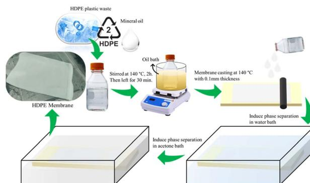
Fig. 1 Preparation scheme of the HDPE membrane.
