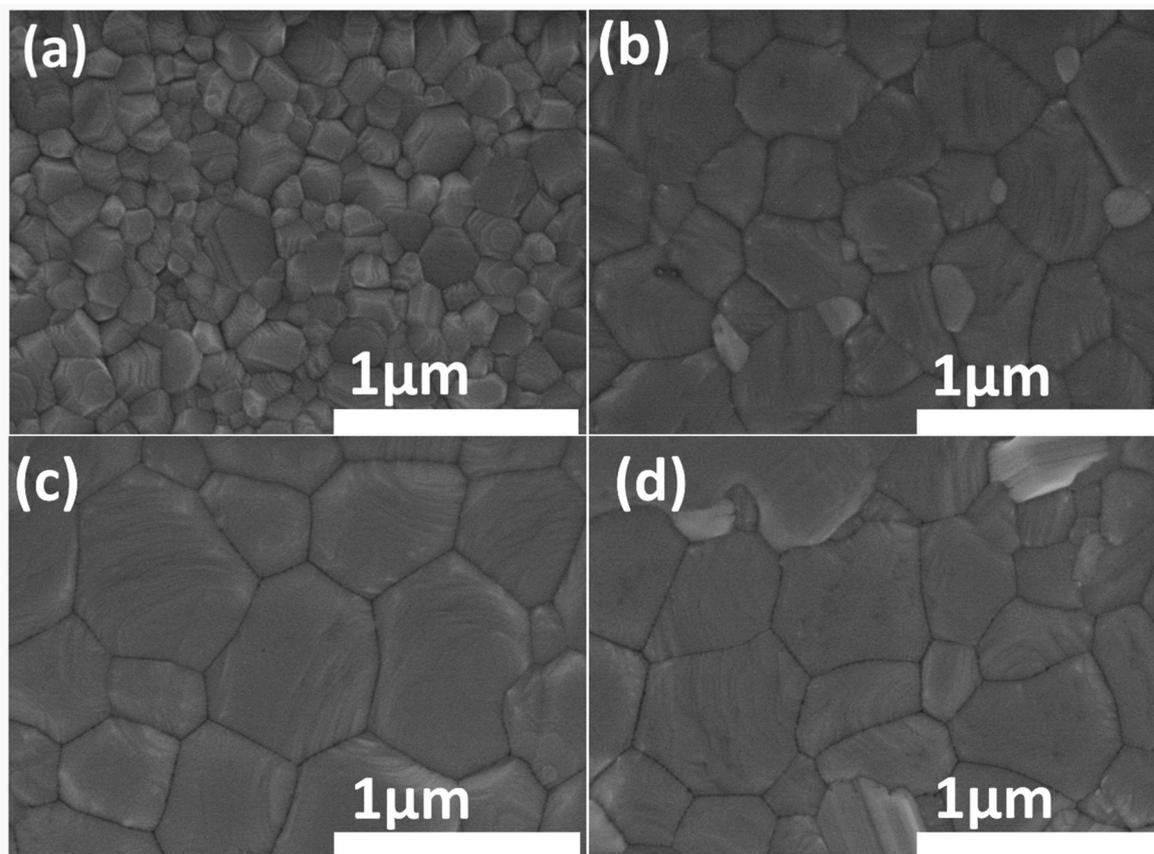
**Fig. 3** Surface scanning electron microscopy (SEM) images of the perovskite intermediate adduct modification equipped with varying concentrations of FAI: (a) 0 mg mL<sup>-1</sup> FAI, (b) 10 mg mL<sup>-1</sup> FAI, (c) 20 mg mL<sup>-1</sup> FAI, and (d) 30 mg mL<sup>-1</sup> FAI.
