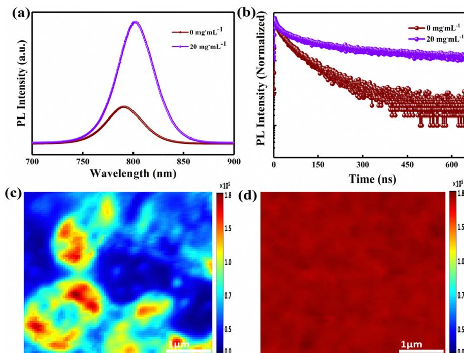
Fig. 5 (a) Steady-state PL spectra and (b) TRPL spectra of control and  $20 \text{ mg mL}^{-1}$ -FAI-based perovskites deposited on the substrate of glass. PL spectral intensity mapping images of (c) control and (d)  $20 \text{ mg mL}^{-1}$ -FAI-based films on the glass substrates.
