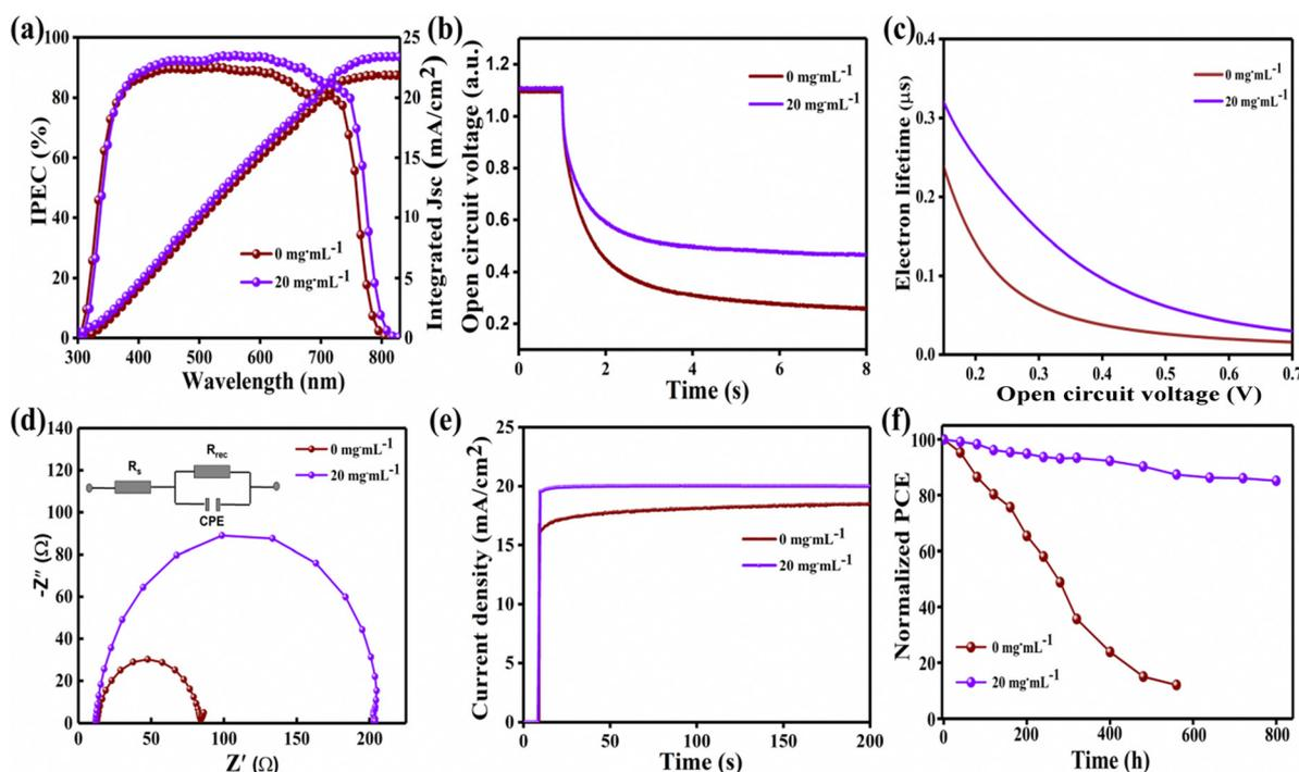
**Fig. 7** Comparisons of the control and 20 mg mL<sup>-1</sup>-FAI based devices: (a) IPCE spectra, (b) transient photo-voltage decays, (c) electron lifetime and  $V_{oc}$  correlation, (d) electrochemical impedance spectroscopy (EIS) with Nyquist plot, (e) stabilized current density at the maximum power point (MPP), and (f) normalized PCE attenuation under 30% relative humidity and 25 °C for about 800 h.
