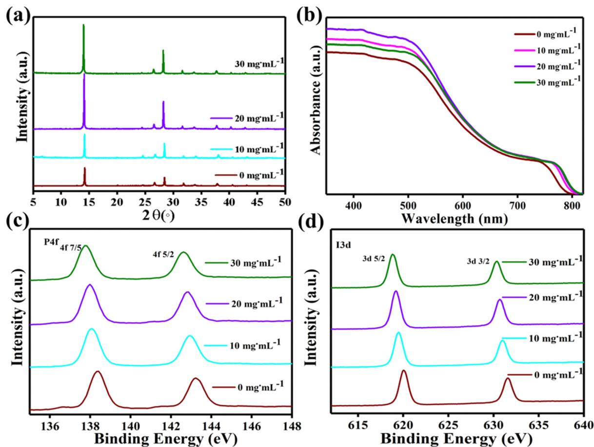
Fig. 4 (a) X-ray diffraction patterns and (b) UV-Vis spectra of the control and FAI-based films with FAI concentrations ranging from 0 mg mL<sup>-1</sup> to 30 mg mL<sup>-1</sup>. XPS spectra of 0 mg mL<sup>-1</sup> to 30 mg mL<sup>-1</sup> FAI-doped perovskites after annealing: (c) Pb 4f and (d) I 3d core spectra of the perovskites with various FAI concentrations.
