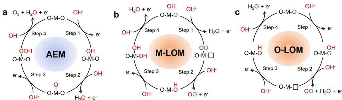
Fig. 3 Schematic OER mechanisms on perovskite oxides: (a) AEM, (b) M-LOM, and (c) O-LOM.
