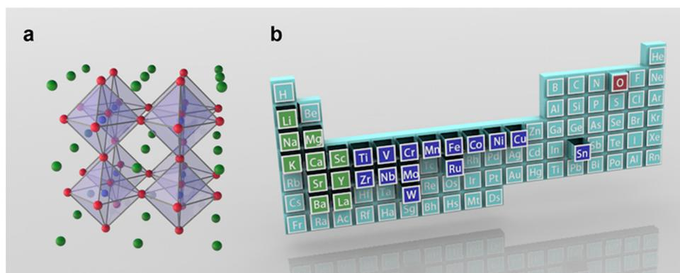
Fig. 2 (a) Schematic illustration of the structure for perovskites (ABO<sub>3</sub>). (b) The commonly used element in perovskite oxides. Green is the A-site element, blue is the B-site element, and red is oxygen.
