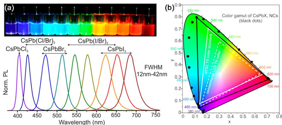
**Fig. 3** (a) PL spectra and photographs of CsPbX<sub>3</sub> (X = Cl, Br, and I) MHP nanocrystals; (b) color coordinates of CsPbX<sub>3</sub> (X = Cl, Br, and I) MHP nanocrystals and the conventional LCD TV color and NTSC TV color standard. Adapted from ref. 3 with permission. Copyright 2015, American Chemical Society.
