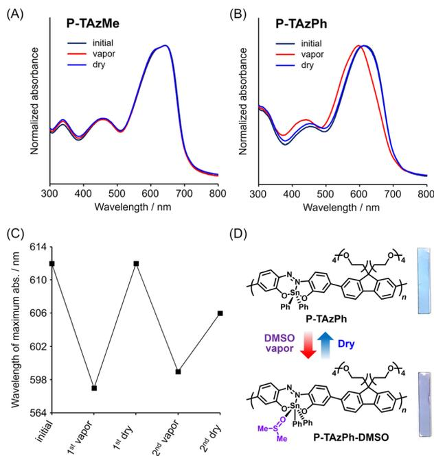
**Fig. 3** UV-vis absorption spectra of (A) **P-TAzMe** and (B) **P-TAzPh** in the film before and after solvent annealing for 30 min, and recovery test by drying the film for 30 min at room temperature. (C) Reversible controls of the UV-vis absorption properties of **P-TAzPh** with exposure to DMSO vapor (30 min) and dry (30 min) processes at room temperature. (D) Illustration of plausible mechanism of vapochromism in the film with photographs under room light.
