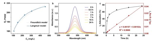
Fig. 5 (a) Langmuir and Freundlich model fitting of the isotherm of iodine adsorption by VMOC-6 in cyclohexane solution. (b) Time evolution of the UV-vis absorption spectra of cyclohexane solutions in the presence of VMOC-6. (c) The kinetics of the adsorption process of iodine on VMOC-6 was plotted with the relative removal rate (%) of iodine (black line) and  $t/Q_t$  (red line) versus time.
