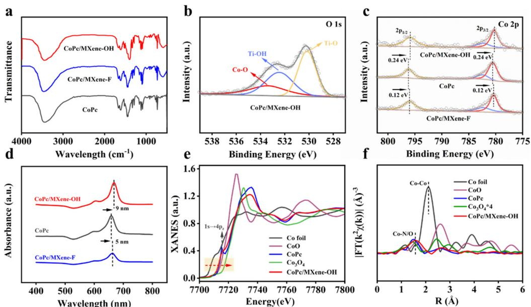
**Fig. 2** (a) FTIR patterns of CoPc, CoPc/MXene-F and CoPc/MXene-OH. (b) O 1s XPS spectrum of CoPc/MXene-OH. (c) Co 2p XPS spectra of CoPc, CoPc/MXene-F and CoPc/MXene-OH. (d) UV-vis spectra of CoPc, CoPc/MXene-F and CoPc/MXene-OH. (e) XANES spectra of CoPc/MXene-OH and comparison samples (Co foil, CoO, Co<sub>3</sub>O<sub>4</sub> and CoPc). (f) EXAFS spectra of CoPc/MXene-OH and comparison samples.
