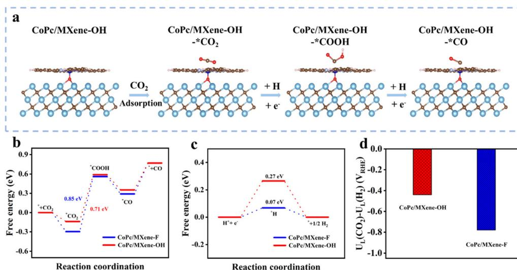
**Fig. 4** (a) The optimized configurations of the adsorption of intermediates on CoPc/MXene-OH. (b) Calculated free energy diagram of CoPc/MXene-F and CoPc/MXene-OH for the ECRR. (c) Calculated free energy diagram of CoPc/MXene-F and CoPc/MXene-OH for the HER. (d) Limiting potential differences between  $\text{CO}_2$  reduction and  $\text{H}_2$  evolution on different catalyst models at  $U = 0 \text{ V}$ .
