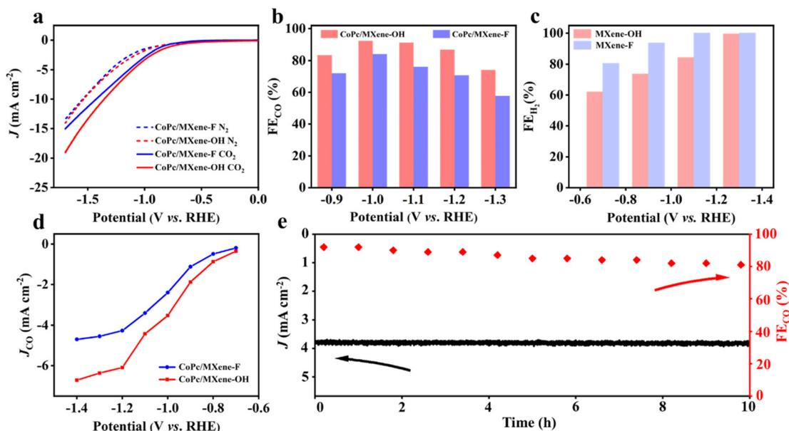
**Fig. 3** (a) LSV curves of CoPc/MXene-F and CoPc/MXene-OH in CO<sub>2</sub>- and N<sub>2</sub>-saturated 0.1 M KHCO<sub>3</sub> solution. (b) FE of CO at various potentials of CoPc/MXene-F and CoPc/MXene-OH. (c) FE of H<sub>2</sub> at various potentials of MXene-F and MXene-OH supports. (d) J<sub>CO</sub> at various potentials of CoPc/MXene-F and CoPc/MXene-OH. (e) Long-term stability at -1.0 V.
