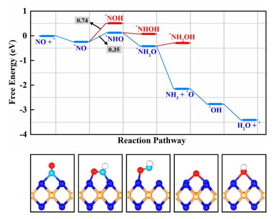
Fig. 4 The energetically most favorable free energy profile for the electroreduction of NO molecules to  $NH_3$  product on the  $\beta$ -PdBi<sub>2</sub> monolayer and the involved reaction intermediates. The blue, orange, red, light blue, and white spheres represent the Bi, Pd, O, N, and H atoms, respectively.
