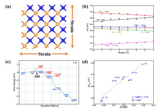
Fig. 6 (a) Schematic of the  $\beta$ -PdBi<sub>2</sub> monolayer under biaxial tensile strain; (b) the relationship of  $\Delta G$  with the strain; (c) the energetically most favorable free energy profile for the electroreduction of NO molecules to the NH<sub>3</sub> product on the β-PdBi<sub>2</sub> monolayer after applying 7% tensile strain and (d) the correlation of the adsorption energy ( $\Delta E_{ads}$ ) of \*NO species with the integrated crystal orbital Hamilton population (ICOHP).
