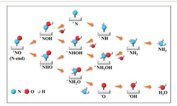
Fig. 3 Schematic depiction of all possible pathways for electrocatalytic NORR to  $NH_3$  along the N-end pathway on the  $\beta$ -PdBi<sub>2</sub> monolayer.
