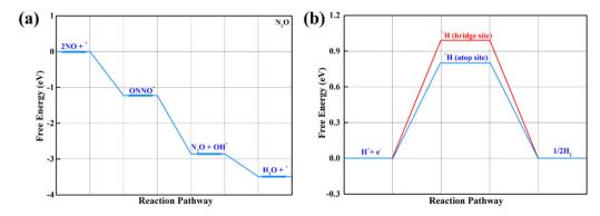
Fig. 5 (a) The energetically most favorable free energy profile for the electroreduction of 2NO molecules to the  $N_2O$  product on the β-PdBi<sub>2</sub> monolayer and (b) the calculated Gibbs free profile of HER on the β-PdBi<sub>2</sub> monolayer.
