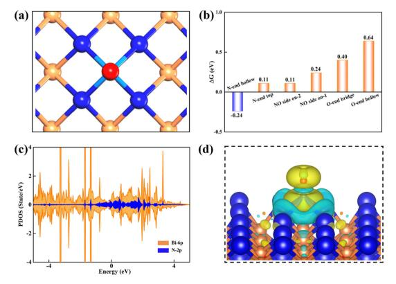
Fig. 2 (a) The optimized configuration, (b) the adsorption free energies ( $\Delta G$ ) for NO adsorption on the  $\beta$ -PdBi<sub>2</sub> monolayer in various possible adsorption patterns, (c) the projected density of states (PDOS) and (d) the charge difference density of the β-PdBi<sub>2</sub> monolayer with an isovalue of  $0.003 \text{ e Å}^{-3}$  (before and after NO adsorption). Cyan and yellow bubbles represent positive and negative charges, respectively.
