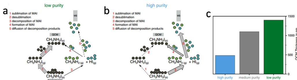
**Fig. 8** Schematic of sublimation and decomposition processes. For low purity MAI (a), the main path (thick arrows) is the sublimation and desublimation. For high purity MAI (b), the main path is the decomposition into methylamine and hydrogen iodide. (c) Comparison of the peak areas extracted for each material. Reproduced with permission.<sup>103</sup> Copyright 2022, Wiley-VCH.
