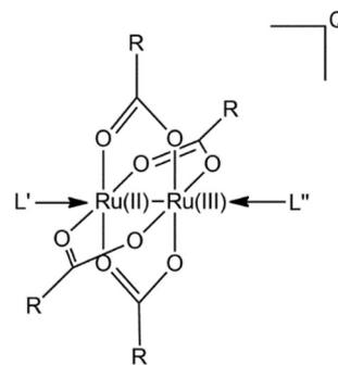
**Fig. 1** General structure of Ru(II)Ru(III) paddlewheel complexes. R-COO<sup>-</sup> = carboxylate ligand; L', L'' = chloro, aquo, hydroxo ligand, and total charge Q.
