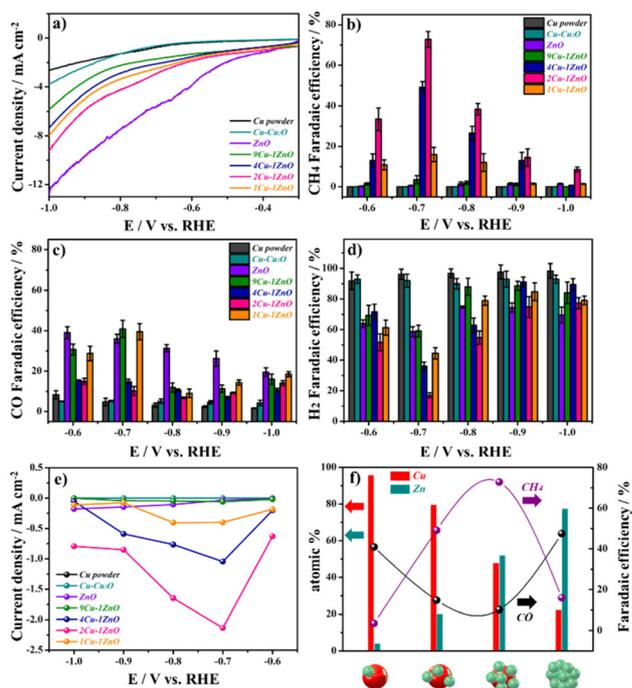
**Fig. 3** (a) Linear sweep voltammetry curves, (b) CH<sub>4</sub> faradaic efficiency, (c) CO faradaic efficiency, and (d) H<sub>2</sub> faradaic efficiency of Cu powder, Cu–Cu<sub>2</sub>O, ZnO, and Cu–ZnO with different Cu : Zn ratios. (e) CH<sub>4</sub> partial current density of different catalysts. (f) Relationship between the performance, components, and morphology of Cu–ZnO catalysts.
