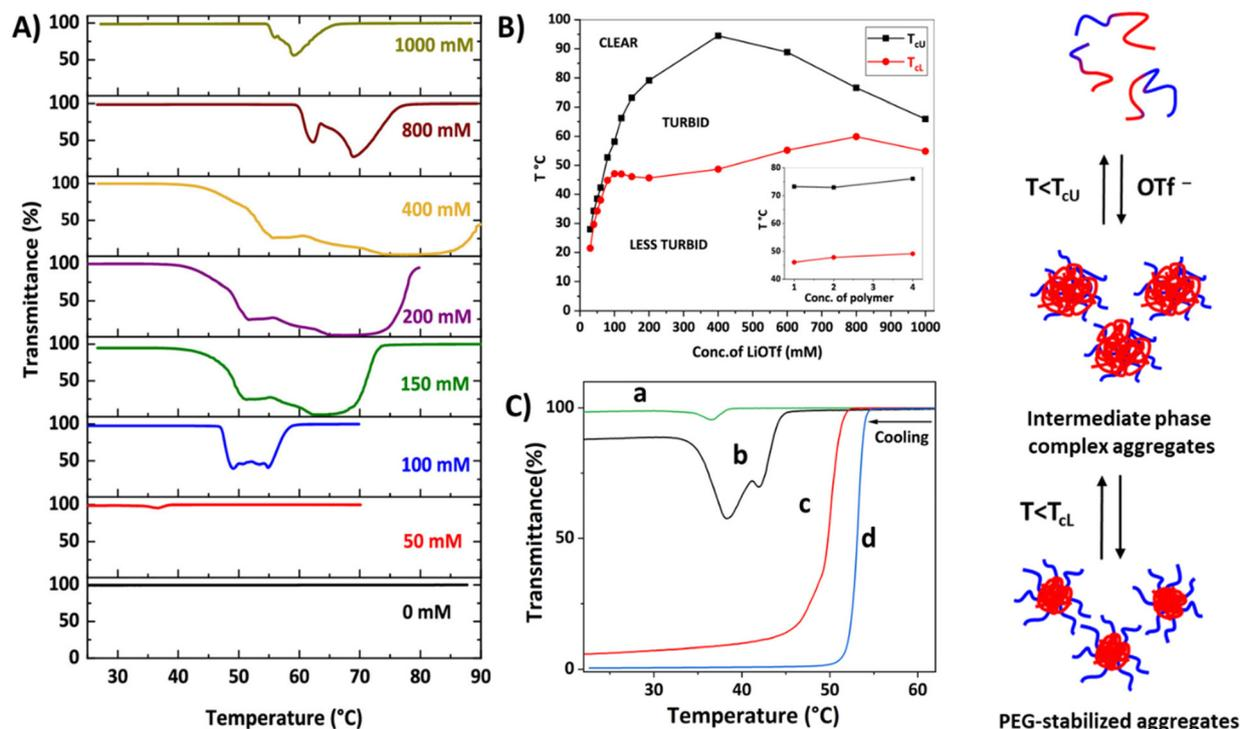
**Fig. 16** (A) Transmittance cooling curves for **P50a** solutions (PVBTMAC DP = 62) and (B)  $T_{CU}$  and  $T_{CL}$  at different polymer concentrations. (C) Transmittance cooling curves for **P50** in aqueous triflate solutions (50 mM LiOTf). PVBTMAC DP ( $a = 62$ ,  $b = 81$ ,  $c = 172$  and  $d = 270$ ). Illustration of PEG-polycation phase separation in aqueous triflate solutions. Reproduced from ref. 141. Copyright 2018 American Chemical Society.
