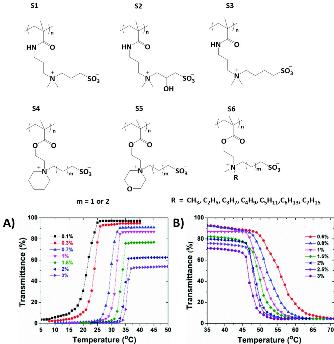
Fig. 2 Series of zwitterionic polysulfobetaines. (A) Transmittance data collected upon cooling S6 with methyl substituents; (B) collected upon heating S6 with a *n*-pentyl substituent at various polymer concentrations. Reproduced from ref. 64. Copyright 2018 Royal Society of Chemistry.
