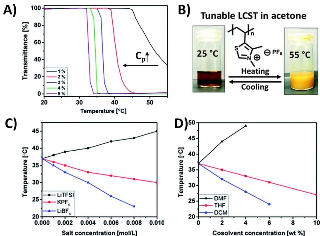
**Fig. 8** (A) Turbidity curves for acetone solutions of **P13** measured at various polymer concentrations. (B) Photographs of a 3 wt% **P13** solution in acetone below the  $T_c$  (left) and above the  $T_c$  (right).  $T_{\text{CL}}$  measured for 3 wt% **P13** solutions in acetone: (C) at different concentrations of external salts; (D) at different concentrations of cosolvents. Reproduced from ref. 100 with permission from the Royal Society of Chemistry, copyright 2016.
