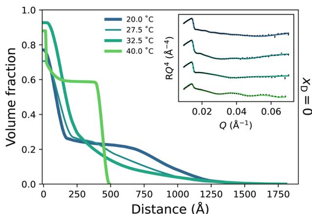
**Fig. 2** Polymer volume fraction profiles of a PNIPAM brush as a function of temperature in D<sub>2</sub>O. Thicker curves represent the VF profiles corresponding to the most swollen, partially collapsed and most collapsed structures. Inset presents corresponding reflectivity and models.
