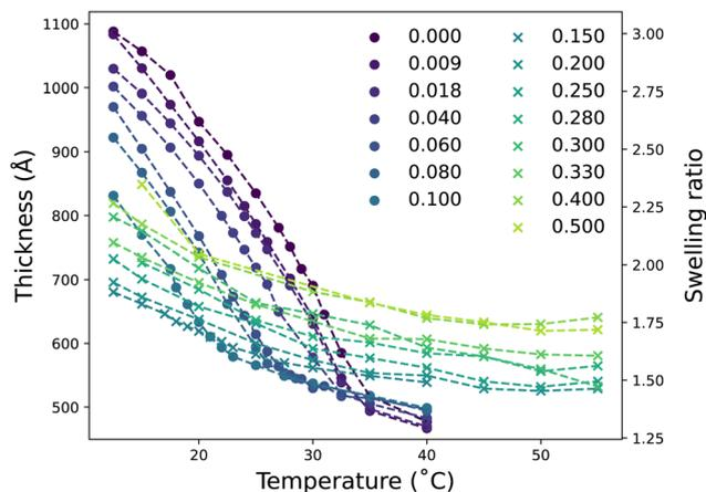
Fig. 1 Ellipsometry determined thickness and swelling ratio of a PNIPAM brush as a function of  $x_D$  and temperature. Circle symbols (●) denote solvent compositions where a clear thermotransition is observed; crosses (×) denote compositions with a severely suppressed thermotransition.
