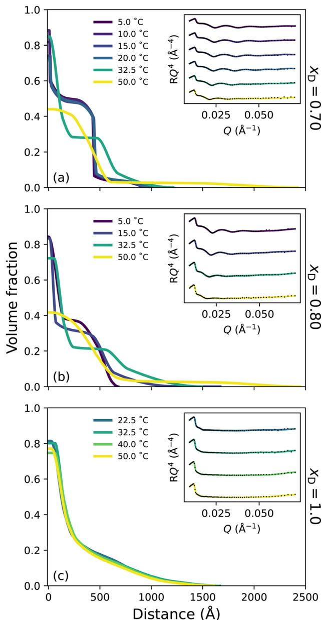
**Fig. 5** Polymer volume fraction profiles of a PNIPAM brush derived by neutron reflectometry in various solvent compositions of increasing as a function of temperature: (a)  $x_D = 0.70$ , (b) 0.80 and (c) 1.0 (pure DMSO). Inset presents corresponding reflectivity and models.
