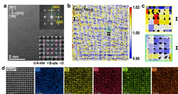
**Fig. 3** (a) HAADF-STEM image along the [100] zone axis for the pyrochlore type (Yb,Tb,Gd,Dy,Er)<sub>2</sub>Ti<sub>2</sub>O<sub>7</sub> HEO with the corresponding FFT pattern in the top inset and the projected structure model in the bottom inset. (b) Lattice strain vectors overlaid on colormaps of the aspect ratios ( $l_{[001]}/l_{[010]}$ ) for all quadrangle units in (a). (c) Enlargements of two types of domains in (b). (d) Atomic-resolution EDS elemental maps of Gd, Tb, Dy, Er, and Yb.
