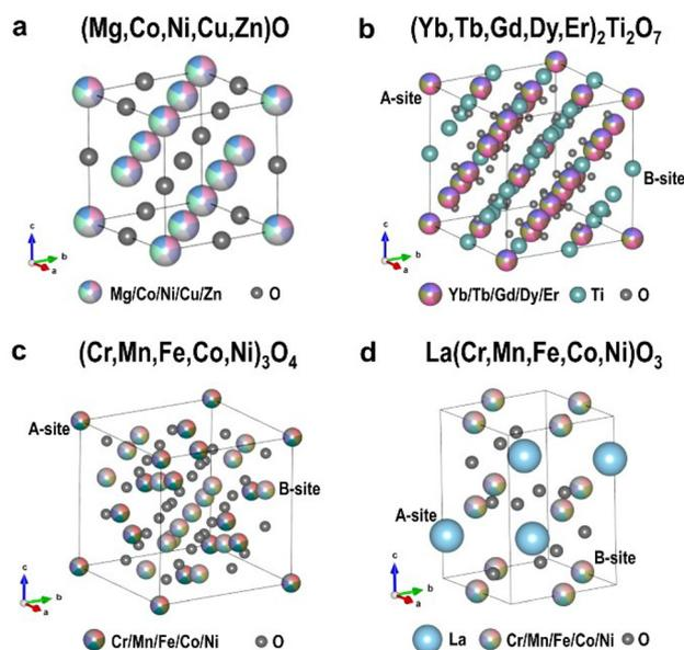
**Fig. 1** Crystal structures of (a) rock-salt type (Mg,Co,Ni,Cu,Zn)O, (b) pyrochlore type (Yb,Tb,Gd,Dy,Er)<sub>2</sub>Ti<sub>2</sub>O<sub>7</sub>, (c) spinel type (Cr,Mn,Fe,Co,Ni)<sub>3</sub>O<sub>4</sub>, and (d) perovskite type La(Cr,Mn,Fe,Co,Ni)O<sub>3</sub>.
