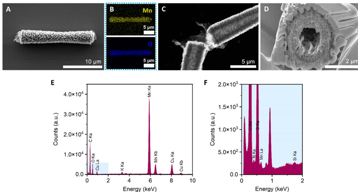
**Fig. 4** Characterization of  $\text{MnO}_2$ /Lac micromotors. (A) High-resolution FESEM image of a  $\text{MnO}_2$  micromotor after the hydrothermal reaction. (B) EDS-mapping of A, showing the Mn (yellow) and O (blue). (C) FETEM image of a  $\text{MnO}_2$  micromotor after laccase immobilization. (D) Cross-section of a  $\text{MnO}_2$  micromotor. (E) Elemental analysis spectrum of a  $\text{MnO}_2$ /Lac micromotor. (F) Magnification of blue square in figure (E) from 0 to 2 keV.
