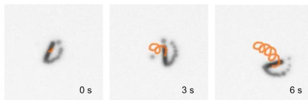
**D** Instantaneous velocities of MnO<sub>2</sub>/Lac micromotors at 2 wt. % H<sub>2</sub>O<sub>2</sub>
