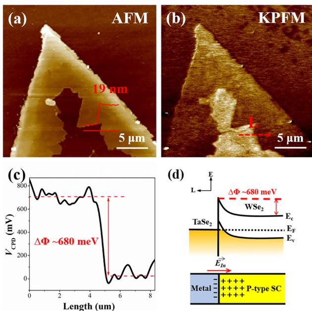
**Fig. 3** (a) AFM topography image and height profile of a representative 2D TaSe<sub>2</sub>-WSe<sub>2</sub> heterostructure. (b) KPFM surface potential maps of a transferred 2D TaSe<sub>2</sub>-WSe<sub>2</sub> heterostructure on a conductive Si substrate. (c) Contact potential difference along the red dashed line in (b). (d) Corresponding schematics of the band profiles for the 2D TaSe<sub>2</sub>-WSe<sub>2</sub> heterostructure according to KPFM characterization.
