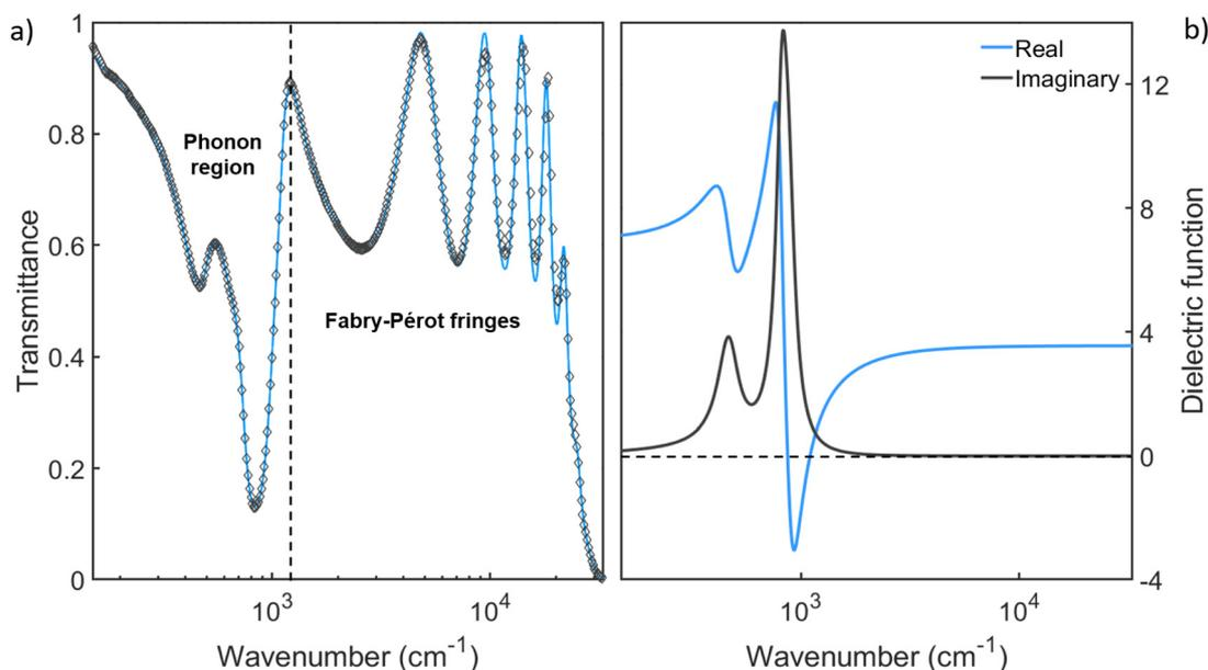
**Fig. 1** (a) Experimental (light blue line) and fitted (black empty diamond symbols) transmittance of the  $\text{Si}_3\text{N}_4$  membrane, measured in the THz-UV range. The vertical black dashed line separates the phonon absorption region (low-frequency) to the high-frequency part characterized by Fabry-Pérot fringes. (b) Real (light blue line) and imaginary (black line) parts of the dielectric function, extracted from the fitted transmittance by considering the Fabry-Pérot effect.
