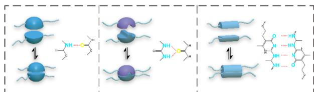
Fig. 2 The three typical hydrogen bonds in PU.
