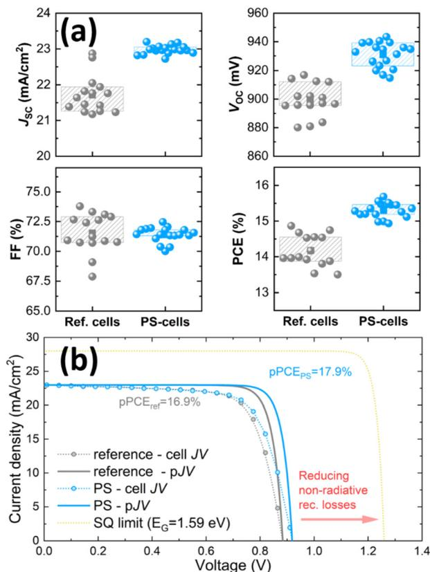
**Fig. 4** (a) Short-circuit current density ( $J_{SC}$ ), open-circuit voltage ( $V_{OC}$ ), fill factor (FF) and power conversion efficiencies of manufactured CPSCs with and without a sacrificial PS layer. (b)  $JV$  curves and pseudo- $JV$  curves of the optimum reference and nano-architected cells, in comparison with the curve at the Shockley–Queisser limit.
