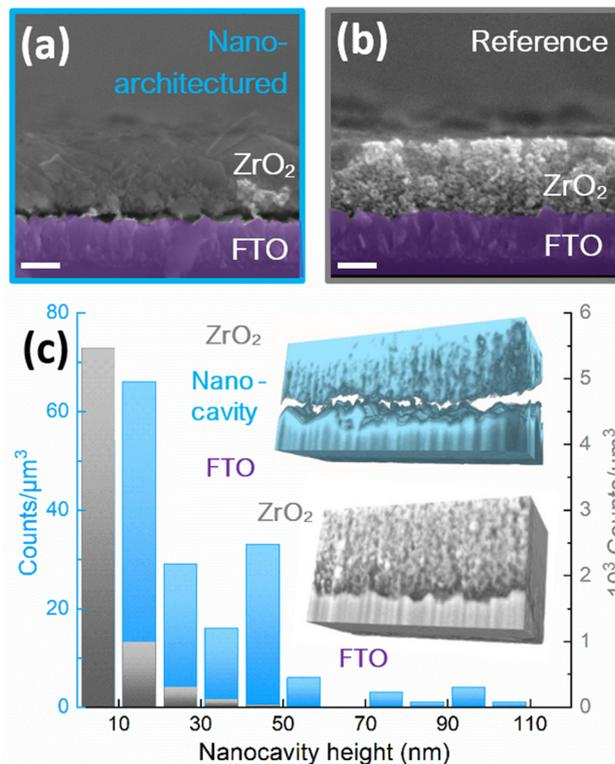
**Fig. 2** Cross-sectional scanning electron microscopy (SEM) images of (a) the nano-architected layer of  $\text{ZrO}_2$  and (b) the reference layer of  $\text{ZrO}_2$ . Scale bars – 500 nm. (c) Distribution of the cavity height in the nano-architected (blue) and reference (grey) samples, obtained from 3D-nanotomography using focused ion-beam (FIB) ablation.
