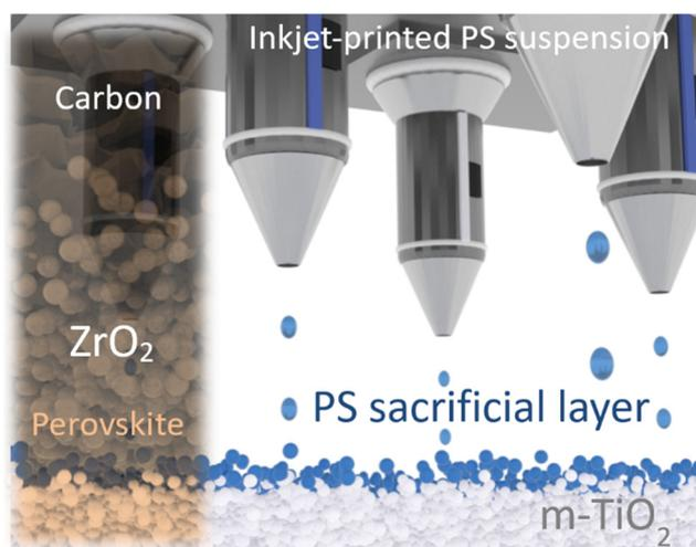
**Fig. 1** Conceptual illustration depicting an inkjet-printing process of a sacrificial layer of polystyrene (PS) particles for nano-architected perovskite solar cells with carbon-based electrodes with a solar cell structure depicted on the left.
