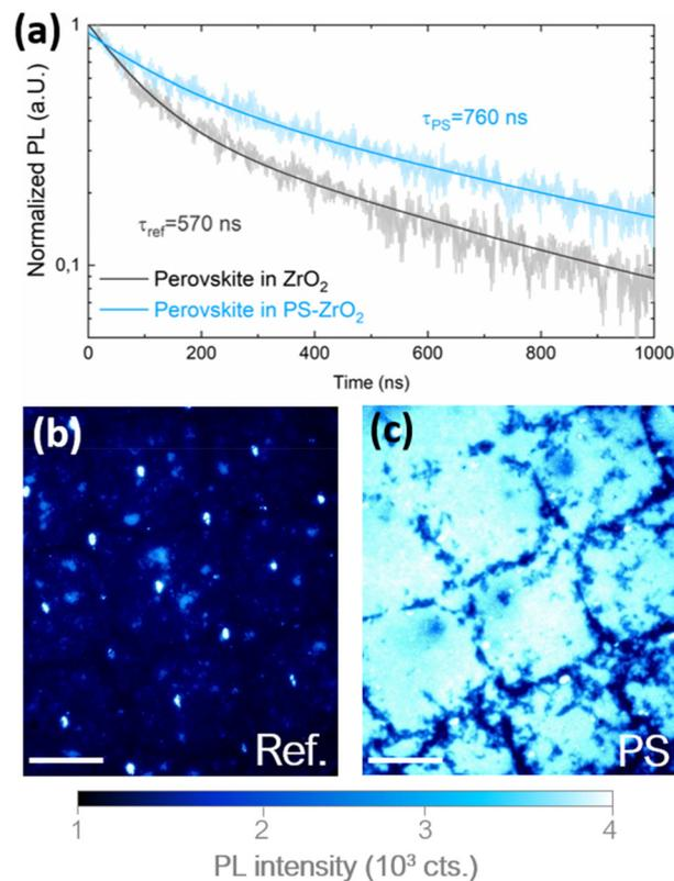
**Fig. 3** (a) Time-resolved photoluminescence (TRPL) measurements of the perovskite embedded in reference  $\text{ZrO}_2$  and nano-architected  $\text{ZrO}_2$  (PS- $\text{ZrO}_2$ ), showing a difference in the decay constant and charge-carrier lifetime. Steady-state PL maps of (b) reference perovskite solar cells with carbon electrodes and (c) nano-architected cells with a PS sacrificial layer. Scale bar – 150  $\mu\text{m}$ .
