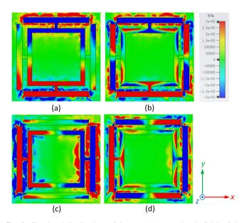
Fig. 4 Simulated distributions of the z-component electric fields of the proposed metamaterial absorber unit cell at resonant frequencies. Distributions at (a) 0.89 THz and (b) 1.36 THz under normal TF polarized incidence. (c) and (d) Distributions at 0.89 THz and 1.36 THz under normal TM polarized incidence, respectively.
