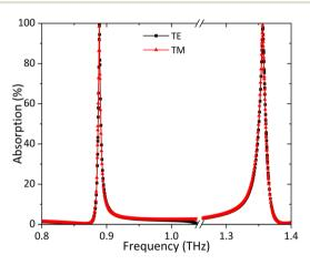
Fig. 2 Absorption spectra of the dual-band metamaterial absorber.
