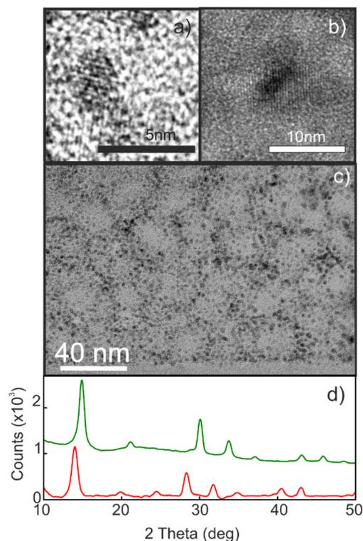
**Fig. 1** (a and b) High-resolution TEM micrographs of MAPbBr<sub>3</sub> (a) and MAPbI<sub>3</sub> (b) nanocrystals inside a porous silica matrix. (c) The TEM cross section of the QD-MAPbBr<sub>3</sub>@SiO<sub>2</sub> composite layer. (d) XRD diffractograms of QD-MAPbBr<sub>3</sub>@SiO<sub>2</sub> (green line) and QD-MAPbI<sub>3</sub>@SiO<sub>2</sub> (red line). For the sake of clarity, backgrounds were subtracted in both diffractograms.
