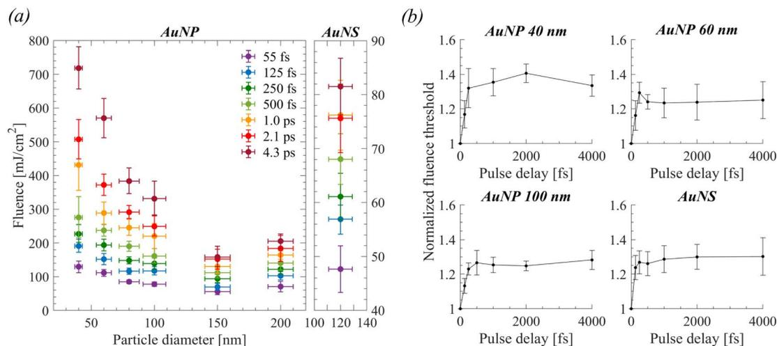
**Fig. 3** (a) Size-dependent, experimentally evaluated fluence thresholds of detectable cavitation bubbles of spherical AuNPs (left) and the ones of AuNS (right) for all applied laser pulse widths. (b) Results of double 55 fs pulse experiments as a function of pulse delay. All fluence thresholds have been normalized to the one acquired under single 55 fs pulse excitation.
