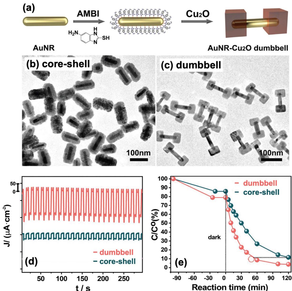
Fig. 7 (a) Schematic diagram of the AMBI-mediated synthesis of dumbbell-type Au–Cu<sub>2</sub>O nanocomposites. (b and c) TEM images of the structures obtained (b) without AMBI and (c) in the presence of AMBI. (d and e) Comparison of the (d) photocurrent response and (e) photocatalytic activity for MO degradation of dumbbell and core–shell structures. Reproduced with permission from ref. 92. Copyright 2023 Wiley-VCH.
