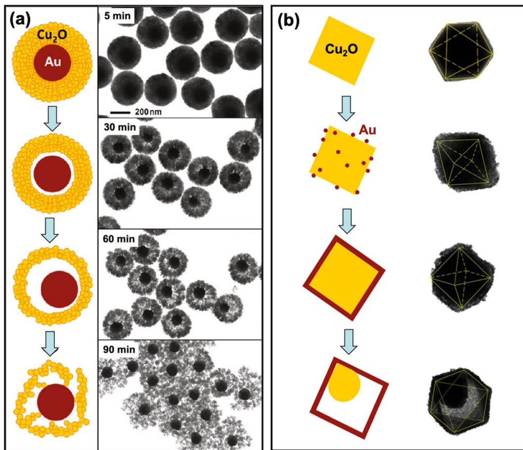
Fig. 5 Schematic representation of the formation of (a) Au@Cu<sub>2</sub>O and (b) Cu<sub>2</sub>O@Au yolk-shell nanocomposites. The TEM images of the structures produced are also shown. Adapted with permission from (a) ref. 80, copyright 2011 American Chemical Society, and (b) ref. 84, copyright 2017 Springer Nature.
