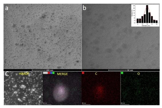
Fig. 1 TEM micrographs and dark-field HAADF-STEM images of CNPs obtained by the hydrothermal treatment of *Madhuca longifolia* flower: (a) lower magnification, (b) higher magnification and inset particle size distribution plot and (c) STEM and EDS mapping.
