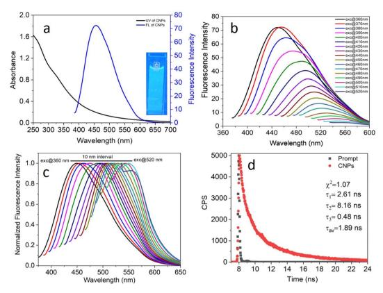
Fig. 3 (a) UV-visible absorption and emission spectra with the inset showing blue fluorescent image ( $\lambda_{ex} = 370$  nm and  $\lambda_{em} = 455$  nm), (b) excitation-dependent emission spectra of CNPs, (c) normalized emission spectra of CNPs in an aqueous medium [CNPs] = 2.0 mg mL<sup>-1</sup> and (d) time-resolved fluorescence decay of CNPs ( $\lambda_{exc} = 405$  nm and  $\lambda_{emi} = 490$  nm).
