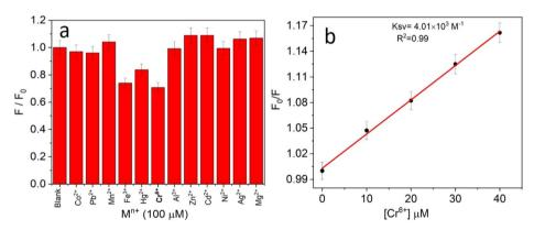
Fig. 5 (a) Fluorescence intensity ratio plot for CNPs in the presence of other heavy metal ions with p-value < 0.05. (b) Calibration plot, CNPs  $(2.0 \text{ mg mL}^{-1})$  against  $\text{Cr}^{6+}$   $(0-10 \, \mu\text{M})$  ion concentration for the estimation of LOD in the aqueous solution [standard deviation =  $\pm 0.043$ , [ $M^{n+1}$ ] = 100  $\mu$ M, [CNPs] = 2.0 mg mL<sup>-1</sup>,  $\lambda_{exc}$  = 370 nm and  $\lambda_{emi}$  = 454 nm].
