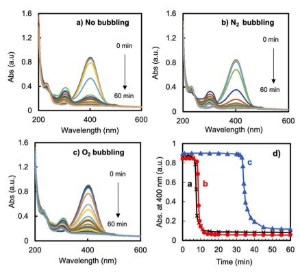
Fig. 4 Reduction of 4-nitrophenol catalyzed by LCCV@AuNP in aqueous solution with a feed ratio of [Au]/[4-NP]/[NaBH<sub>4</sub>] = 1/1.71/1693 ([Au] =  $0.021 \, \mu$ mol mL $^{-1}$ ). (a–c) UV-vis spectra of the reaction recorded at fixed time intervals. (d) Plots of the absorbance at 400 nm at different reaction times from the spectra in (a–c).
