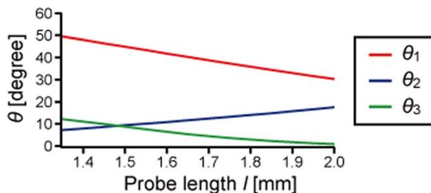
Fig. 5 The tip oscillation angle of the first (red), second (blue), and third (green) eigenmodes,  $\theta_i = \arctan |A_v/A_l|$ , for the properties listed in Table 1 while varying the probe length.  $\theta_1$  is relatively close to 90° (normal to the surface).  $\theta_2$  and  $\theta_3$  are relatively close to 0° (parallel to the surface).
