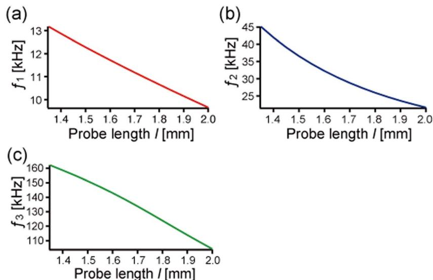
Fig. 3 The first three eigenfrequencies calculated by using the properties listed in Table 1 while varying the probe length. (a) The first eigenfrequency,  $f_1$ . (b) The second eigenfrequency,  $f_2$ . (c) The third eigenfrequency,  $f_3$ .
