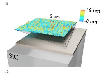
Fig. 5 Fabricated samples. (a) Photos of the samples with increasing Ti film thickness, deposited on top of a 220 µm SiC wafer. (b) Detail of a 25 μm<sup>2</sup> roughness of the selected sample (20 nm Ti thin film) measured via AFM. The RMS roughness is 2.188 nm, mean roughness is 1.635 nm, maximum peak height is 16.05 nm, maximum pit depth is 7.73 nm and the maximum height is 23.78 nm.
