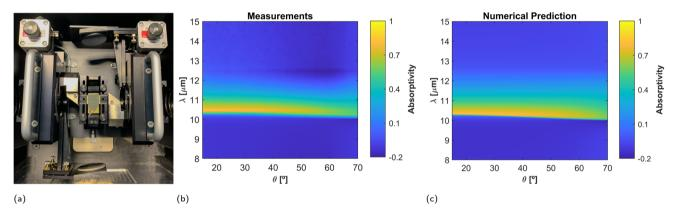
Fig. 8 Oblique incidence measurements. (a) Photograph of the moving mirror setup for adjusting the incident angle. Comparison between (b) measurements and (c) numerical predictions of the film absorptivity as a function of the incidence angle, for the sample of 20 nm film thickness. Measurements were performed from 15° to 80° with a step of 1°.
