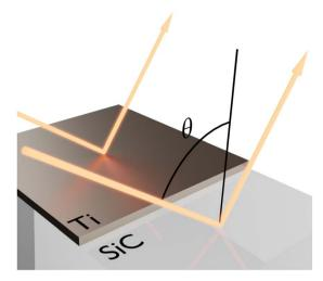
Fig. 6 Reflectivity difference. Representation of reflectivities involved in the subtraction: thin film plus substrate  $(R_{TiSiC})$  and the substrate itself ( $R_{SiC}$ ), for a determined incidence angle ( $\theta$ ).
