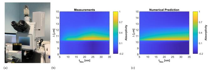
Fig. 7 Normal incidence measurements. (a) Photograph of the FTIR microscope. Comparison between (b) measurements and (c) numerical predictions of the reflectivity difference as a function of the titanium (Ti) film thickness at normal incidence. Measurements were performed on six samples with Ti film thicknesses of 5 nm, 10 nm, 15 nm, 20 nm, 25 nm and 35 nm.
